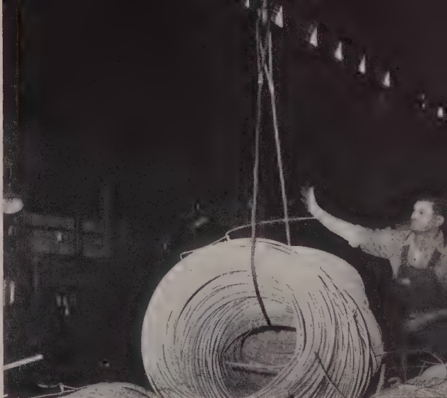
A Gary plant uses Red-Strand single-part slings for many lifting jobs like this. These slings are available with various combinations of end fittings for attaching the sling to rings or lugs. Single-part slings frequently are the most economical to use.
