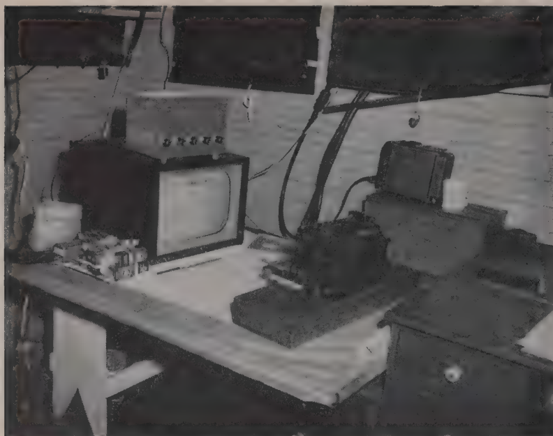
PORTABLE TV RECEIVER used as monitor had a camera located in front of it to make permanent record. An observer watching screen would direct operating personnel over an intercom system.
