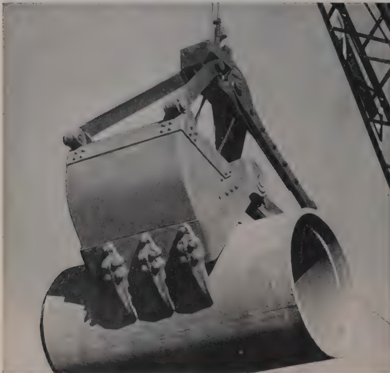
On the job photo shows an ERIE bucket's no-slip grip on concrete pipe being moved at Edward J. Petrillo, Inc. on the New York Thruway.
