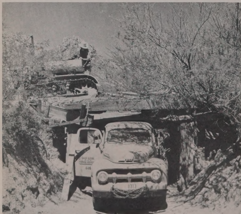
LOADING UP, twice during an ordinary day, Smith pilots an old Cat Thirty, bulldozing decomposed granite through the trap into his truck bed.
