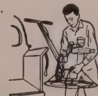
Midget Trowel. New. Lightweight, one man carries; gets into tight spots; only 24" across yet does top trowel job 6 times as fast as by hand. 70 lbs.; 1.6 hp engine.
