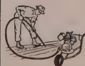
Concrete Vibrator. 9,000 rpm vibration, yet lightweight; rugged, gives long service; gas and elec.; wheel mounting available; accessory tools; 1 1/2 to 6 hp power units.
