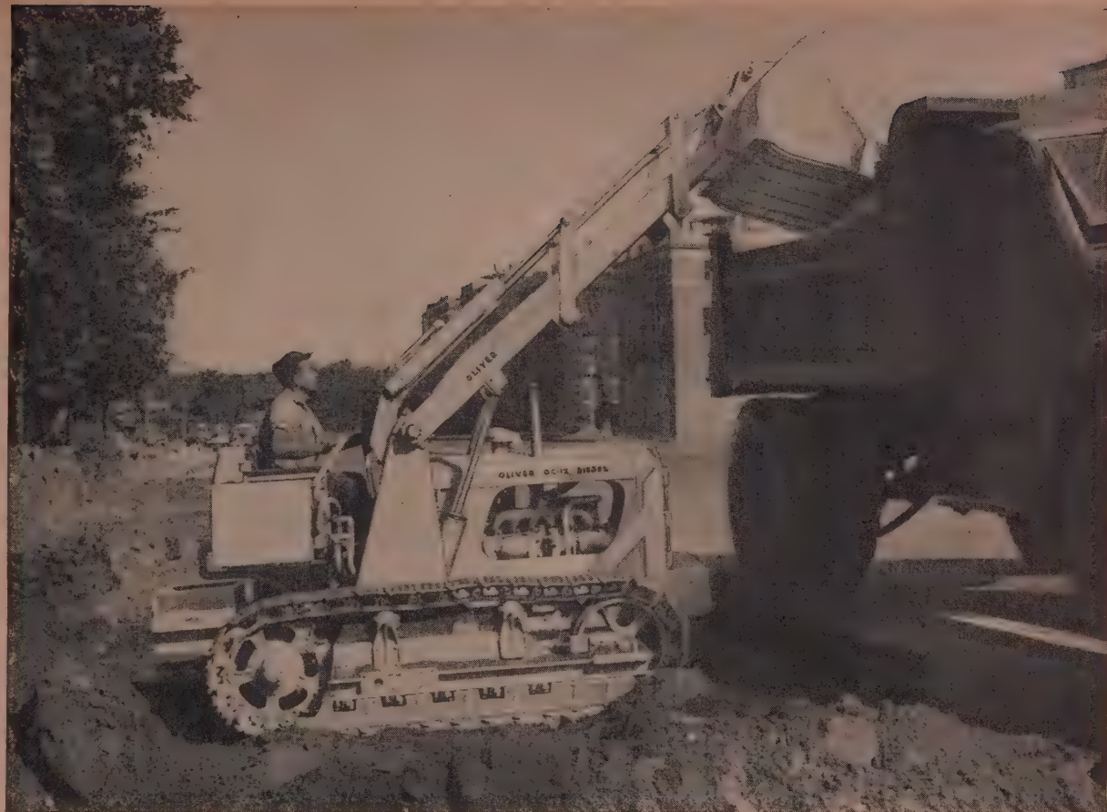
Oliver "OC-12" with hydraulic 1 1/4-yd. loader. This model has the long track frame for added stability. Loader has exceptional bucket rotation and 10' 4" loading height.
