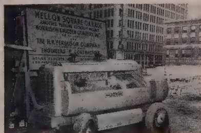
This "315" powers paving breakers on a Pittsburgh construction job.
