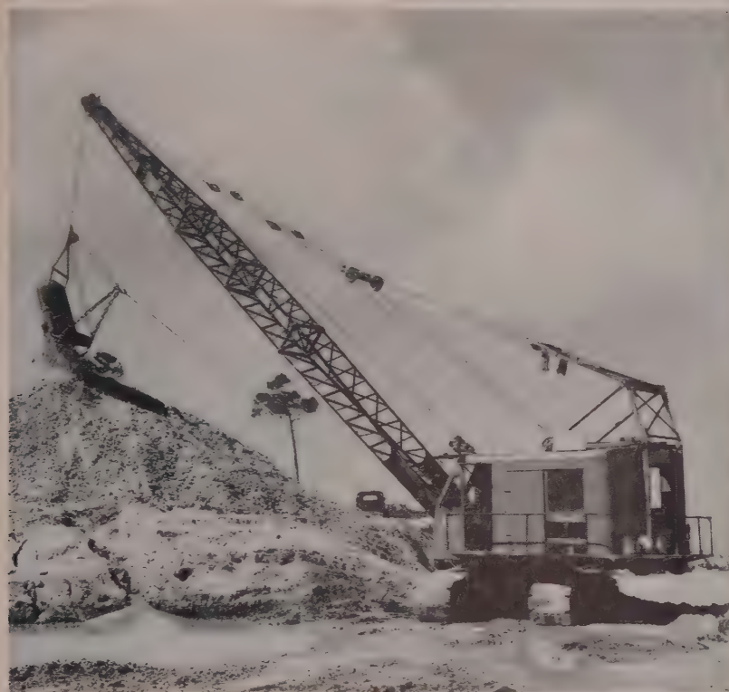
AS A 1¾-YARD DRAGLINE. This fast swinging K-375 rig digs coral rock and sand in Florida. Speed-o-Matic control makes dig-swing-dump one fluid motion because operator has perfect "feel" of the load. There are no grabby clutches that produce lag and lost motion.
