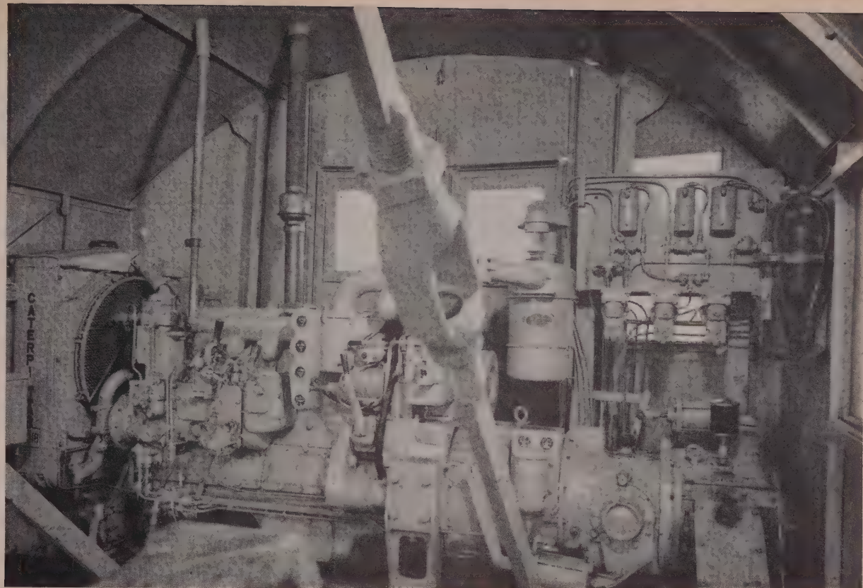
This Caterpillar D318 Diesel—powering a crane—works through a Twin Disc Model CF Torque Converter which provides faster work cycles, protects both engine and driven equipment. Behind the Model CF are a Twin Disc Reverse Gear and two Twin Disc Heavy-Duty Friction Clutches.
