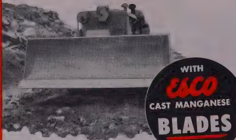
Like all ESCO blades, this sectional ESCO Dozer Blade is cast of special work-hardening manganese steel.
