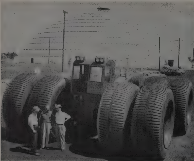
HERE IS 23 Tons that rolls along on a tire pressure of only 5 psi. Each wheel is 10 ft. high and 4 ft. wide. All electric drive system simplified design.
