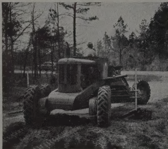
4 Fingertip hydraulic rear steer makes it easy to maneuver around obstructions.
