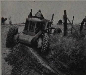
1 All-Wheel Steer carries continuous ditch cuts around corners.
