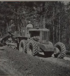
7 Controlled traction moves big windrows, farther and faster.
