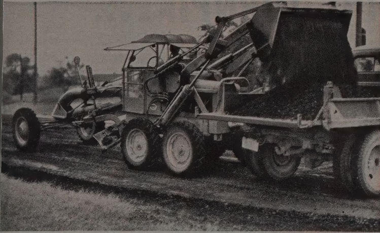
Cleans up, loads trucks with hydraulically operated rear-end loader . . . handles sand, gravel, dirt, any material with \frac{5}{8} -yd bucket.
