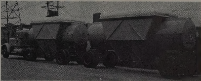
PAYLOAD BOTH WAYS —This truck and trailer hauls a payload of 46,000 lb. of bulk cement from the Oro Grande plant of Riverside Cement Co. to Los Angeles area. An equivalent load of fuel oil is hauled on the return trip. Utility Trailer Manufacturing Co. of Los Angeles designed and engineered the unit in cooperation with Thos. F. Tugwell, Riverside Cement's director of transportation.
