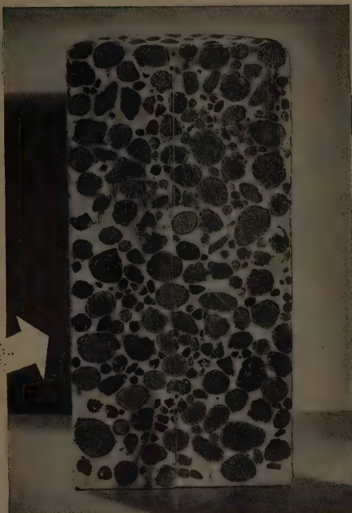
• This cross section of a typical test cylinder of a conventional slump concrete shows the rounded particles, the good gradation and the excellent placement of the material.
