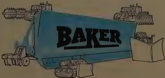
Baker Sectional Tripping feature. Blade swings back over obstruction; snaps back fast into normal position.
