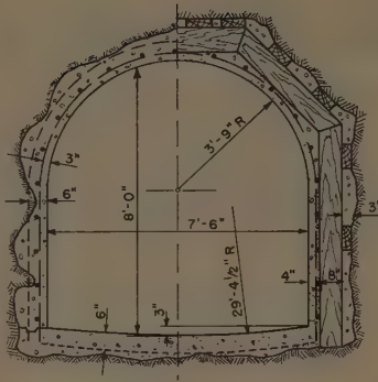
SPECIFICATION AND RESULTS are shown here. Drawing indicates lining for two types of tunnel. Reinforcing steel is placed only as directed—little has been used. Collapsible steel forms establish flat crown, leaving room above for slickline as concrete is placed.
