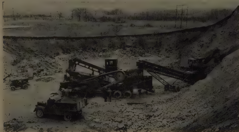
DESIGNED for use in areas where ordinary gravel deposits are becoming depleted is this newest development in portable crushing plants. It produces usable material from large boulders by means of a 3 x 6-ft. scalping screen ahead of an 18 x 30-in. jaw crusher. Sizing and separation are done on a 4 x 10-ft. 1½ deck screen operating ahead of a 30 x 18-in. triple roll crusher.
