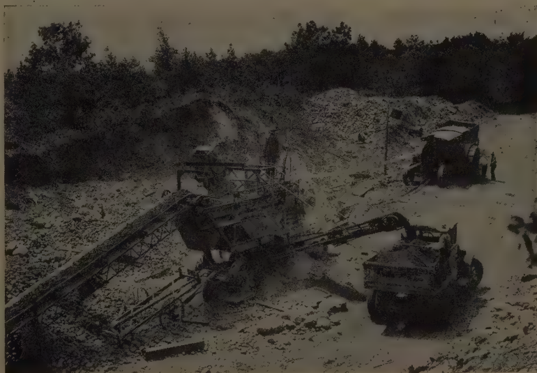
UP TO 500 cu. yd. could be handled in a 10-hr. day in this old Pioneer screening, crushing, and loading Plant No. 12. It cost about $8,000 and weighed 32,350 lb. This pit scene was photographed about 1930.
