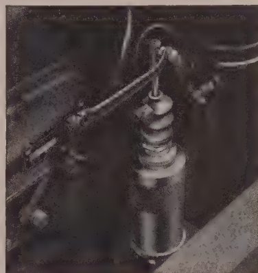
Jaeger "Fuel Miser" standard on all models where automatic control of engine speeds means worthwhile fuel savings.
