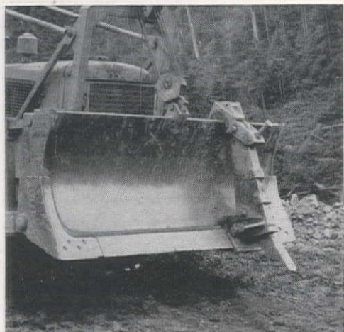
Rooter mounted on dozer blade. Second rooter is usually installed to double effectiveness.
