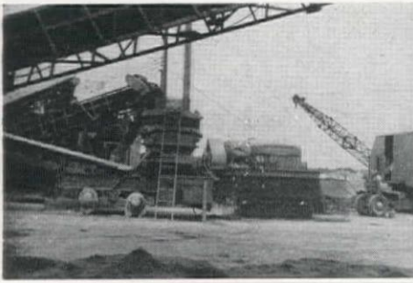
TELSMITH crusher is mounted on frame of 12-in. I-beams, is fitted with dual axle for hauling as a semi-trailer.
