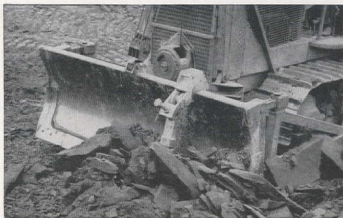
Buck Forte Rooter on a straight dozer rooting unshot sedimentary ocean rock for aggregate plant.
