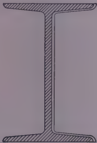
WIDE FLANGE BEAMS
