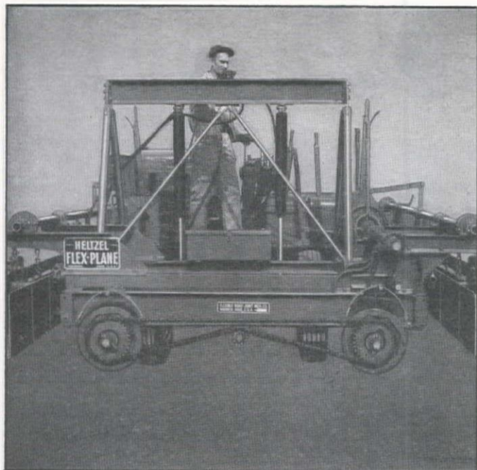
Fastest mobile finisher made today. Screeds slung outside frame enable the Special to hug the forms eliminating swaying and weaving, permitting better surfacing.
