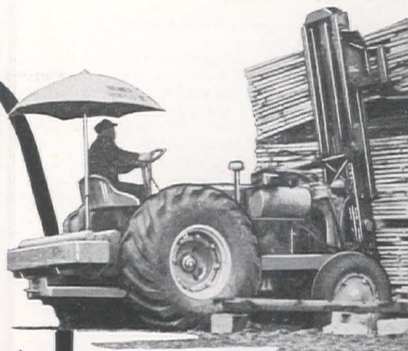
Big lifts of lumber are brought from saw rig to storage yard at Marquette, Michigan. Hydraulically operated loader levels to pick up and put down load, tilts back to carry.
