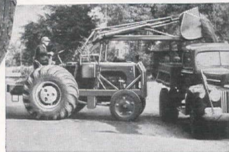
Scraping up cinders and loading them into truck at Stoughton, Wisconsin. Same "LAI" Tractor and loader with hydraulic lift and dump also stock-piles materials, loads trucks during snow removal.
