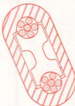
Left: Under pressure, rope retains its round cross section without crushing or distortion, developing over 90% of rated rope strength.
