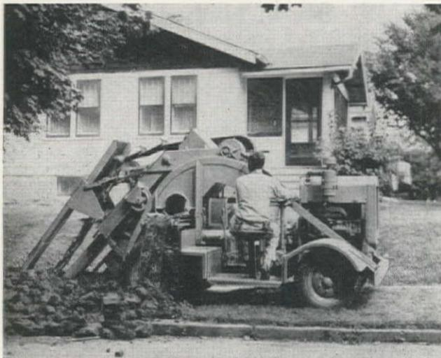
all-welded arch type frame. Variable speed selections are provided for operating the bucket line, conveyor belt, travel and digging traction. The Trenchmobile has road speeds up to 12.65 mph. for self-powered moves between jobs. Pneumatic tire mounting plus low ground pressure permits working and traveling over sidewalks, lawns, without surface damage. Parsons Co., a subsidiary of Koehring Co., is the manufacturer.
