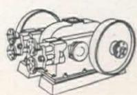
This TRIPLEX TAMPER — three CP pneumatic backfill tamper power units on a Gunderson-Taylor mounting — has 75 square inches of compaction area and enables one man to do the work of five individually operated tampers. Greater thickness of fill can be compacted to specifications; lifts can be increased as much as 20%; compactness is more uniform.
