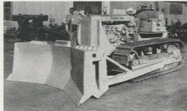
bulldozer for carrying large yardages greater distances, together with the ability to side cast, back fill and pioneer hillside cuts, excavations and roadways by the use of single wing. Users with a regular bulldozer blade can now have the above advantages and can, of course, easily remove the Angle Wing and use the bulldozer as a pusher.
