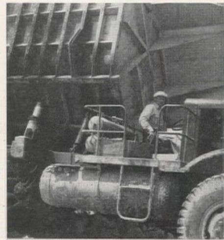
TANK INSTALLED for LP-gas on a 20-*yd.* side-dump truck. These special fuel tanks must be designed for a working pressure of 250 psi.
