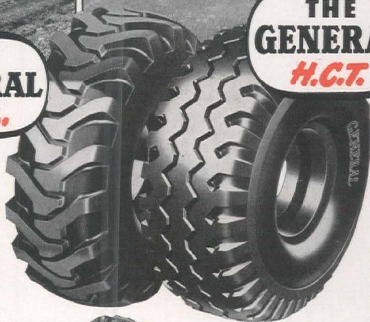
**GENERAL D.T.L.** with deep, sharp, angled cleats and sturdy, high shoulder lugs. Designed for maximum traction on soft surfaces—forward or backward.
