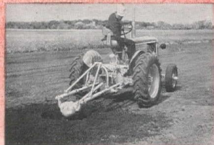
**POST HOLE DIGGER** does the work of eight or ten men. Dig holes for fence posts, tree nursery settings, highway guard-rails, foundation footings and other construction work. Eight auger sizes, 4" to 24" diam.
