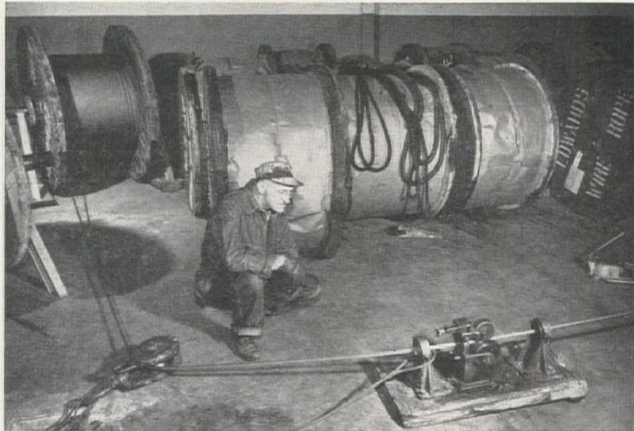
quired to by-pass intervening reels. From the spool and through these blocks, the rope is drawn through a counting machine on the floor by a special winding machine, designed and made in Republic Supply's manufacturing division. On this machine, a delivery spool is placed on a
