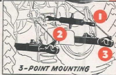
A fast, sure coupling unit for rear-mounted equipment—do ditching, grading, scraping, bulldozing, backfilling, snow handling—dig post holes, remove posts, lift and carry sacks of cement, planks, construction equipment, etc. Many uses on lighter jobs where big, heavy equipment is not needed—also a cost-saver on clean-up and auxiliary work where heavy equipment is on the job.
