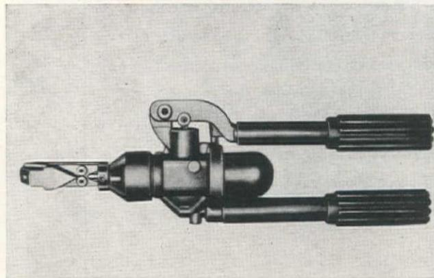
Manco Model 200-A is a pressure of 8,500 psi., exerting 10 tons thrust in a hand operated unit. Also important is a newly designed dual ratio pump which combines rapid traverse with high power to minimize cutting time. Blades, which can be easily resharpened, are alloy steel. The Manco Manufacturing Co. is the manufacturer.
