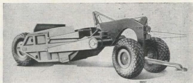
cutting edge. Material is carried in a flat, double-bottom bowl of high tensile steel. Operation is by means of a "Cat" Cable Control unit, which can be mounted on the rear of the tractor to provide positive loading and ejection. Tapered roller bearings are installed at each axle. The scraper uses two 24.00-29 front tires and two 27.00-33 rear tires, all four of 24-ply rating. When loaded, the scraper distributes 60% of the weight on the rear tires. Caterpillar Tractor Co. is the manufacturer.
