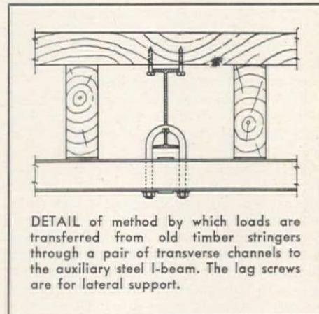
DETAIL of method by which loads are transferred from old timber stringers through a pair of transverse channels to the auxiliary steel I-beam. The lag screws are for lateral support.
