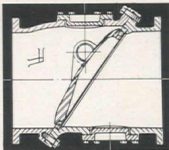
Cross-section of the Chapman Tilting Disc Check Valve. A feature of the design is that the disc seat lifts away from the body seat when opening, and drops into contact when closing, with no sliding or wearing of the seats.
