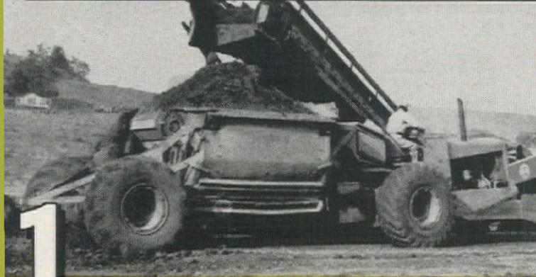
**FASTER LOADING** — Short, wide 9'x11' top opening requires minimum movement, minimum time to "top out" under belt loader. Shovel or dragline operator has easy target, low 8'9" loading height that speeds swing, reduces spillage.
