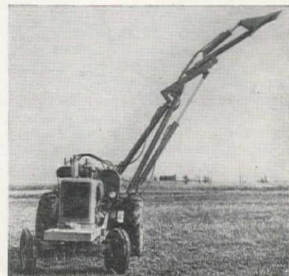
swing, 16-ft. reach and 19-ft. boom-extended height. The digging depth is 9 ft., and the operating pressure is 1,000 psi. The Hopto Digger has a lifting capacity of 2,000 lb., and larger capacities with stabilizers. The completely hydraulic unit has a Vickers and Blackhawk hydraulic system and is manufactured by Badger Machine Co.
