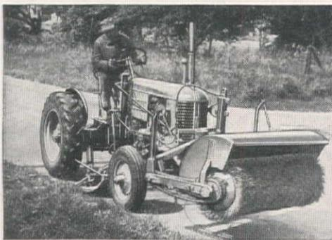
Same man, same "VAI" Case Tractor does mowing or sweeping without waste of time between jobs. Snow plows, blades, scrapers also can be used.
