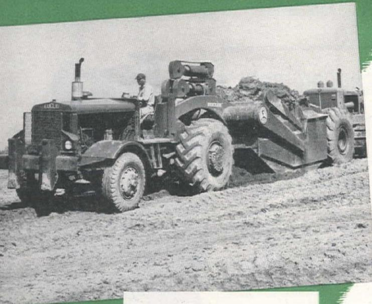
Four wheel Euclid tractor provides easy, positive steering, excellent maneuverability, and has ample power, traction and flotation for fast loading and travel on steep grades and soft fills.
