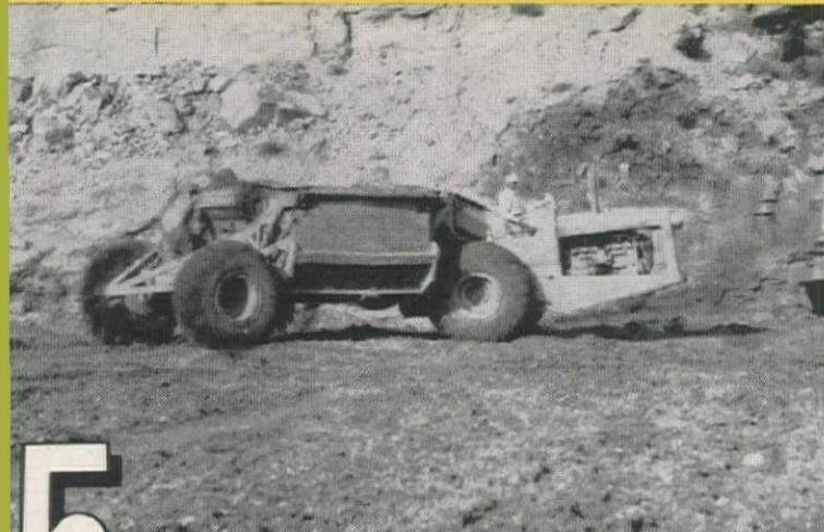
**FAST TURNS OFF FILL** — 25" clearance (with gates open) and 15'8" turn radius permit fast dump and quick turn over windrows even when turning down steep side slopes. You can also back up and swing 90° to clear up to 42" boulders.
