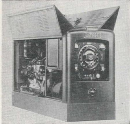
generator controls, meters, welding and ground cable terminals, polarity switch, ignition switch, starter button, etc. The generator is of the symmetrical, 4-pole Multi-Range design. It has 4 laminated main poles and 4 interpoles which are
