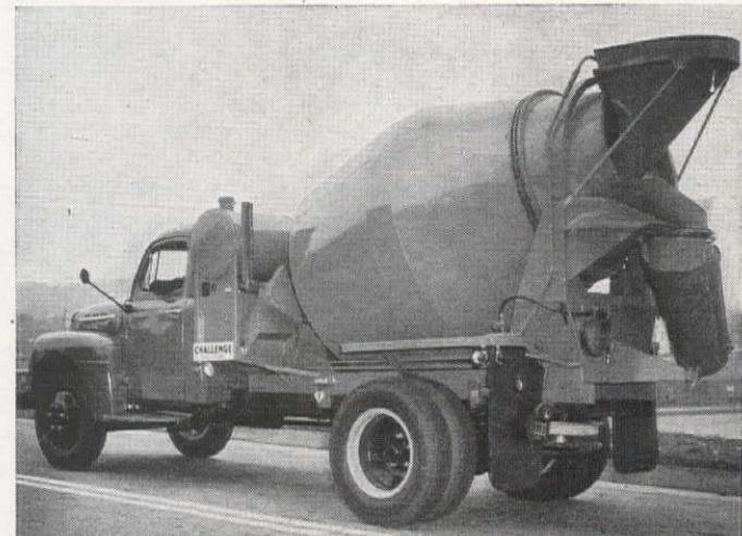
Pictured above is the latest addition to the complete line of Challenge Mixers. This is the 3 1/2-cu. yd. model announced by Cook Bros. Equipment Co. This model is designed and rated to carry 3 1/2 cu. yd. of specification concrete on two-axle trucks.
