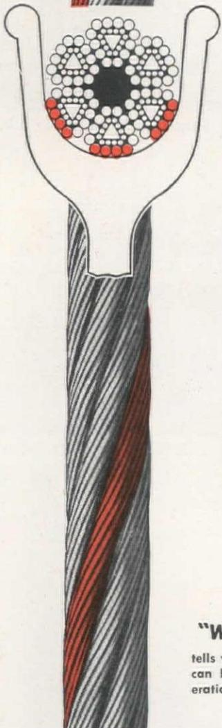
SEE the keystone shape of the strands? Notice how compactly they fit together? That's the answer. There is more steel and less fiber in HERCULES Flattened Strand than in any other wire rope construction of equal size. And if you specify wire rope core, you get still more strength—7½% more—in the same diameter. That extra strength is often mighty useful—safer, too.
