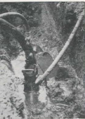
**Dependable Pumping** — with the VP4 Pneumatic Sump Pump. Top-suction prevents clogging — protects motor and bearings from mud.
