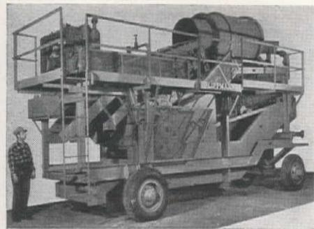
additional strength has been given throughout the plant for even more rugged wear. These improvements have been added without out-of-line price increase. The capacity of this plant runs as high as 80 cu. yd. per hour and it is completely portable for mobile operations. Lippmann Engineering Works is the manufacturer.
