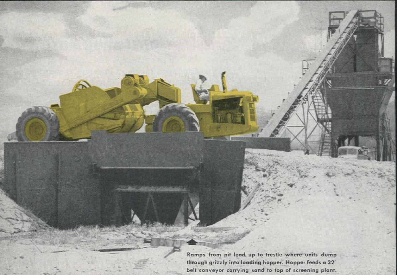
Ramps from pit lead up to trestle where units dump through grizzly into loading hopper. Hopper feeds a 22" belt conveyor carrying sand to top of screening plant.
