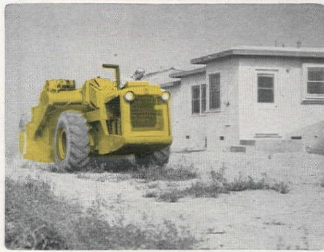
Before renting his Tournapull to Consolidated, Macbeth used the "D" on a series of highway, land leveling, and housing jobs. "It works well in confined places," says Macbeth, "can carry loads over concrete curbing without damage, self-loads well, drives anywhere." On this housing project, it delivered 10 to 11 loads of hard, dry, silty loam hourly over a typical 4400' cycle. Performance was so good on all these jobs that Macbeth recently bought his 2nd D Tournapull!
