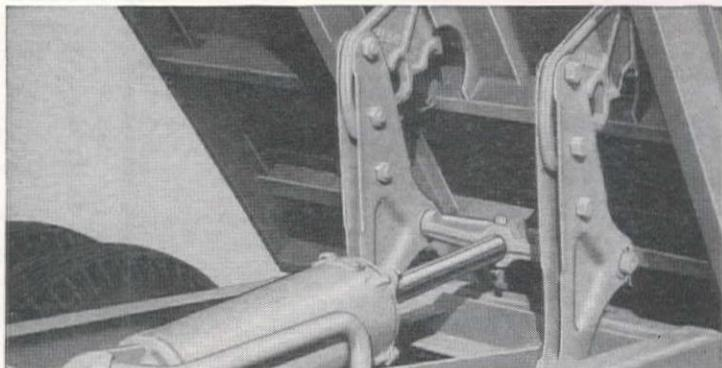
Scientifically positioned fulcrums and transfer linkages automatically "shift" the load at different points, eliminating lift-shock and smoothing out lifting action throughout the dumping cycle. The result is longer hoist, body and chassis life . . . better dumping performance!
