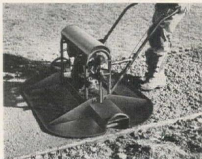
be lost with a hand tamper. The tamper is designed for one-man operation. It has an automatic clutch and governor-controlled speed, adjustable from 500 to 1,500 tamps per minute. Surfaces of all bearings are fully protected from mortar and dust. Two-quart capacity gasoline tank permits continuous operation for four hours without refueling. Float is of abrasion resistant moly steel. Gar-Bro Manufacturing Co. is the manufacturer.
