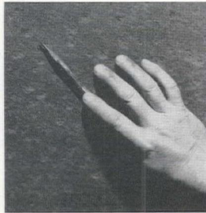
CLEANED steel surface shows the pitting which had developed during ten years of service as a result of corrosion.
