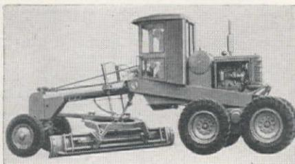
15,000 lb., carry 10- or 12-ft. blade and are perfectly suited for medium class, ditch to ditch service, with 1:1 slopes. Unique feature of these units is that they can be purchased to fit particular job requirements . . . the price depending upon the feature selected (i.e., single or
