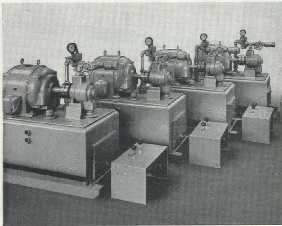
► Hydraulic power units and controls for Lookout Point Dam, designed and built by RUCKER to rotate, raise, return and lock gates of four Walker free discharge valves operating under 200 feet head of water. These units have 20 hp. motors, 25 g.p.m. pumps and deliver 1600 p.s.i. Each operates an 8" diameter, 162" stroke lifting ram, and an 8" diameter, 51" stroke locking and rotating ram. Corps of Engineers job; contractor, Willamette Iron & Steel Company.
