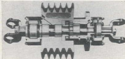
duty truck-mounted equipment. It contains 12 less parts than its predecessor, the Davey 75, and is 25 lb. lighter. Another new feature is a vacuum shift control which is offered as optional equipment. The take-off unit itself is identical for all trucks. The P-80 is 18 in. long and weighs 140 lb.
