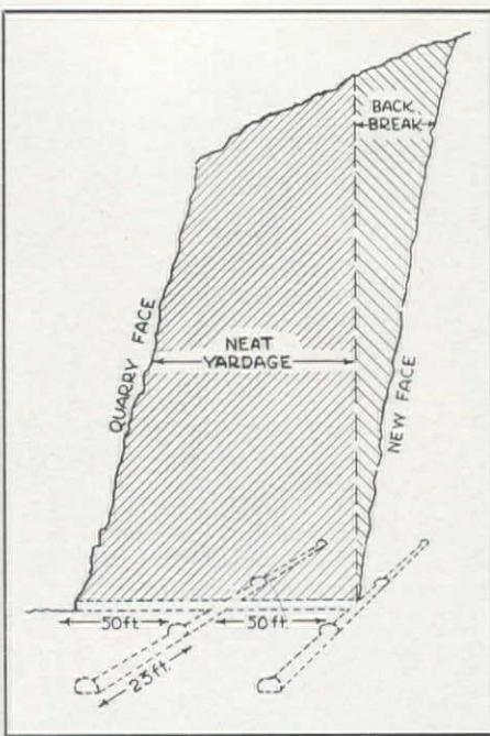
TYPICAL SECTION of quarry face shows general arrangement for a major blast. Maximum height of quarry face last season was 215 ft.
