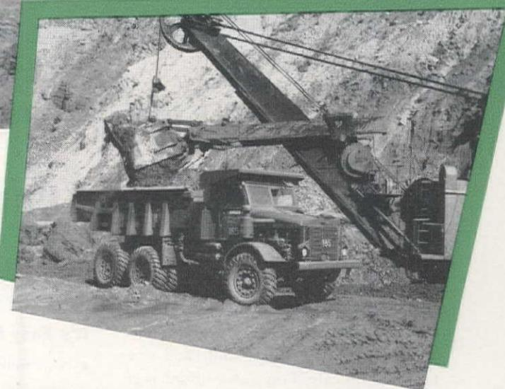
Rear-Dump "Eucs" are designed and built to move rock, coal, ore, overburden and other heavy excavation. They range in capacity from 10 to 34 tons, have top speeds up to 36.3 m.p.h. with full payload, and diesel engines of 125 to 400 h.p.
