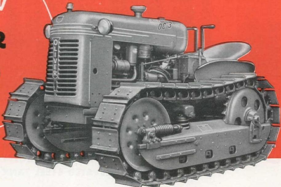
Here's the greatest little crawler tractor you've ever seen . . . the new Oliver Industrial "OC-3". It's ideally balanced for most effective loading and dozing . . . engine is mounted back so that front of tracks and radiator are practically in line. This better balance gives you 40% more lift with a front end loader . . . does a superior job of dozing and grading because blade is mounted close to the tracks for easier handling . . . precise control! And, operators find this bal-
