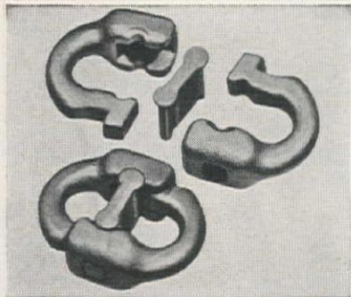
strength of comparable alloy chain. The Wedglok spacer is in compression when the link is carrying a load, and it will not shear or loosen if the projecting spacer points are properly positioned. Only two sizes of Wedglok Universal links are needed to connect any size chain from  $\frac{1}{4}$  in. to  $\frac{3}{4}$  in., depending
