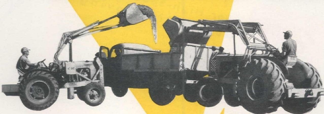
**UTIL** High-turbulence, slow-speed, 51 h.p. engine is the power and economy leader . . . 6 shuttle speeds cut job time . . . 18 roller bearings in steering and front axle assembly for easy handling of capacity front-end loads.
