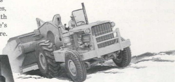
Up a hill on the way to the dirt pit is a Caterpillar DW-20. The 4½-mile trip is made every 20 minutes.
