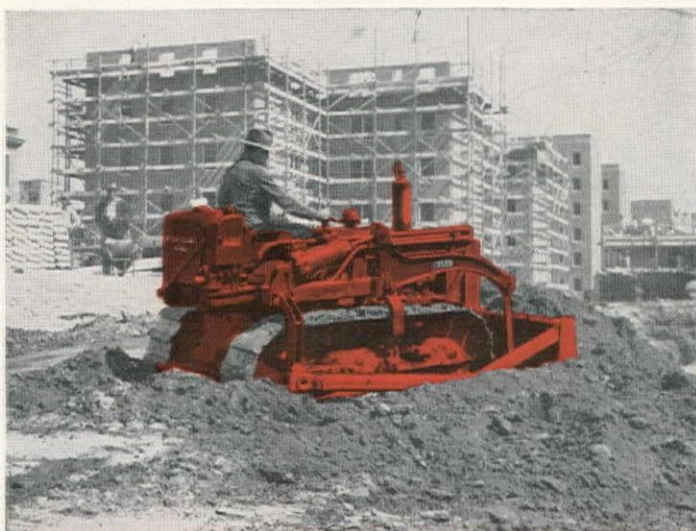
★ This TD-6 bulldozer handles dozens of odd jobs on a construction site. Here it builds a ramp for a housing project in Brooklyn, N.Y.
