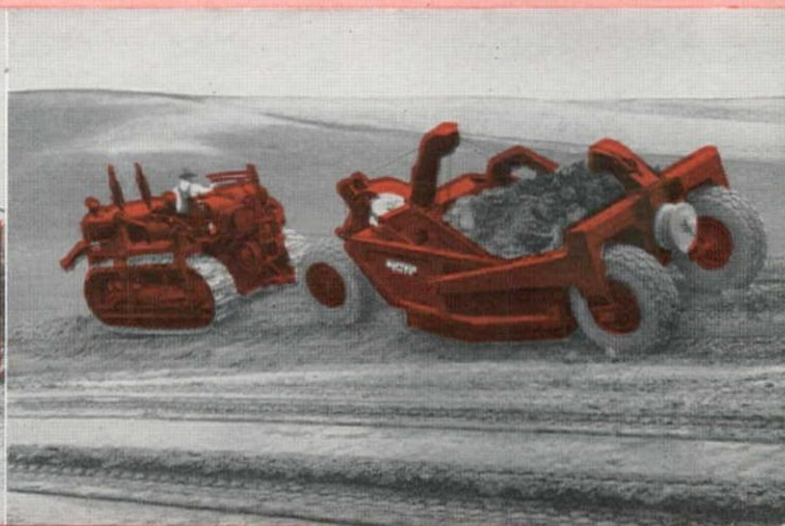
★ Fast loading and easy dumping, with Bucyrus-Erie's exclusive two-part hinged apron, makes this S-91 scraper an ideal tool for road building in Nebraska.
