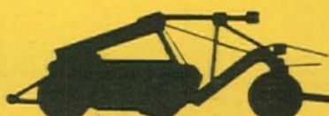
CARRYALL* SCRAPERS capacities from 4 to 23 heaped yards
