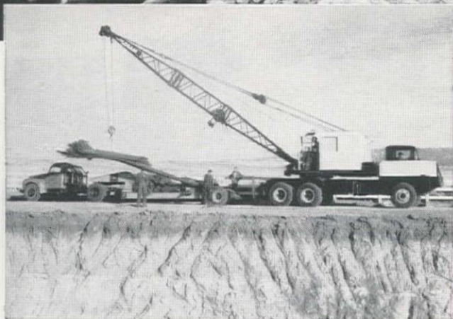
A Lorain MC-504W 25-ton Moto-Crane. It's a basic "50" turntable but with different mounting and front end.
