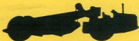
TOURNAPULLS* 7, 14, 27½, 42-yd. capacities speeds, 28 to 35 m.p.h.
