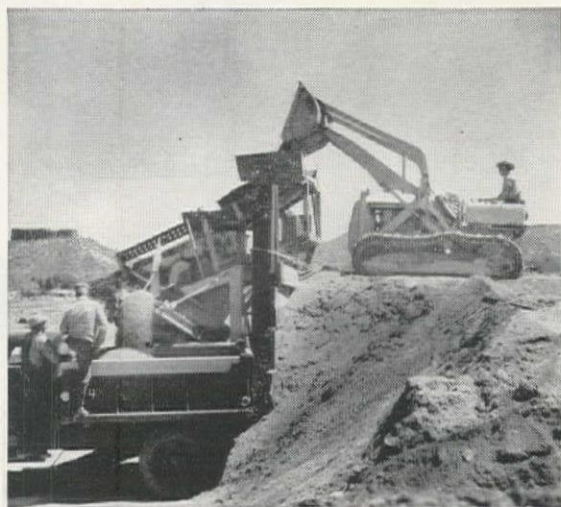
Digging and feeding pit-run gravel to the screen hopper, this hydraulically controlled HT4 TRAXCAVATOR handles over 500 cubic yards a day for Douglas County, Colorado.
