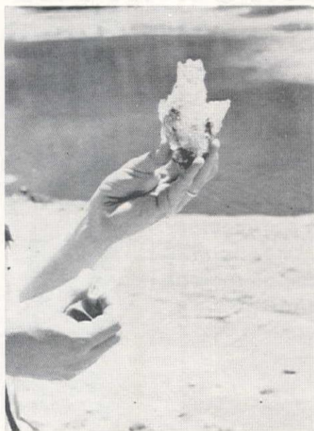
CRYSTALS of sodium carbonate like this formed layer that was several feet thick when flushing began.
