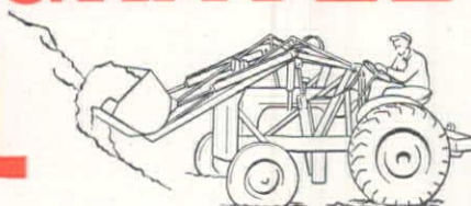
CONSTRUCTION WORK. Case "SI" Tractor completes grading and backfilling work at Bon Ami Homes project in New York. Moves over 200 yards per day.
