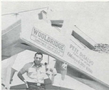
Pete DiSalvo, contractor, is preparing a tract for 1,300 homes at Redwood City, Calif. and using this 17.5-cu. yd. rig. About 500,000 yd. of dirt is to be moved on job.
