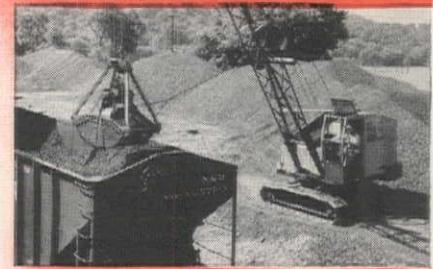
Rapid loading of hopper cars is easily accomplished with this Owen Bucket.
