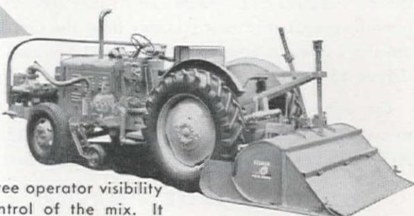
The SEAMAN TRAV-L-PLANT (right) offers all the advantages of the Self-Propelled unit. It is equipped with tachometer assembly and a volumetric meter is available for the closely controlled application of bitumen. Water also is readily applied.
