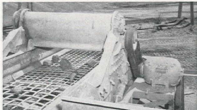
(B) Oversize rocks are removed by this scalping screen at the beginning of the conveyor system. A G-E 20-hp motor operates the screen. Maximum flow of material to the screen comes from an apron feeder operated by a G-E variable speed motor remotely controlled with a rheostat by the operator at the top of the washing plant.
