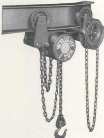
beam sizes, and can be changed from plain to geared or vice versa in a few minutes time as both the plain and geared mountings are identical. The Geared Trolley is constructed like the plain trolley except that the wheels are furnished with gear rings having cut teeth, pinions with cut teeth handwheel, hand chain and hand chain guide. Thrust rollers are mounted to insure proper alignment of the assembly whether on straight or curved track.
