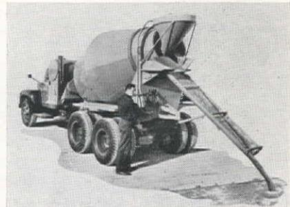
the 6-yr. size (7 1/4-yr. agitator) weighs 6,615 lb., and has a 290-cu. ft. drum volume; and the 6 1/2-yr. size (8-yr. agitator) weighs 7,120 lb., and has a 313-cu. ft. drum volume. Concrete is thoroughly mixed and delivered without segregation right down to the end of the load, regardless of slump.
