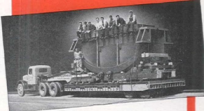
Fruehauf Carryalls are available in capacities from 10 to 74 tons in the standard models . . . to 110 tons in "specials". Frame designs as single- or double-drop "Semi" or full Trailers. No matter what your hauling problem may be, there's a Fruehauf Carryall to fit your job.
