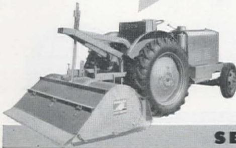
The SEAMAN Self-Propelled (left) is a complete mixing unit which offers full 360 degree operator visibility and accurate control of the mix. It also frees a critical tractor for other work . . .
