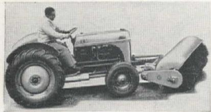
tilts to adjust itself to any surface on which it is applied. There is a full length dust hood over the broom to protect the operator. Broom is driven by rear power take-off at
