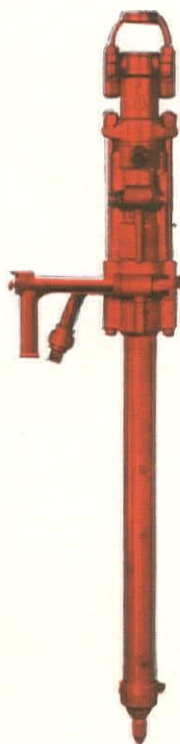
STOPER LEG Converts Sinkers To Stoppers
