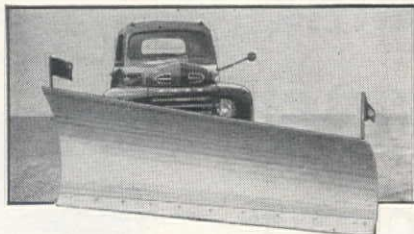
One way plow—Crimped blade means better aeration—sturdy, balanced design.
