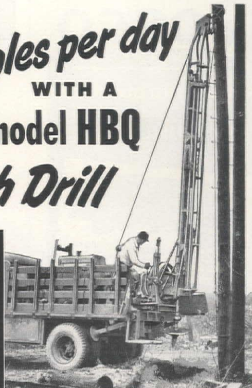
HBQ Tower is quickly, easily positioned hydraulically. Speeds pole setting.
