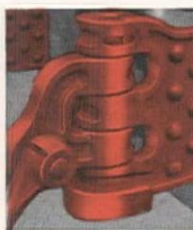
VERTICAL PIN HITCH PLATES. Standard equipment on 5\frac{1}{2} yd. sizes or larger. Optional on others.
