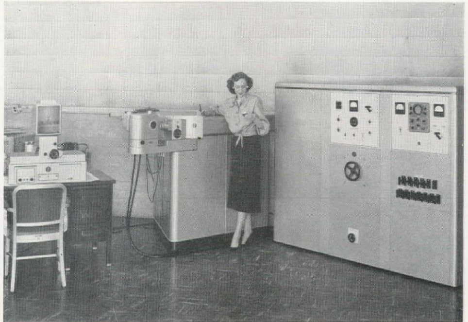
SPECTROGRAPHIC ANALYZER—analyzes cement samples by vaporizing them in the heat of an electric arc, separating their elements into the colors of the spectrum and photographing results for interpretation.
