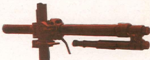
AIR BAR FEED Converts Drifters and Sinkers to Power Feed Drifting
