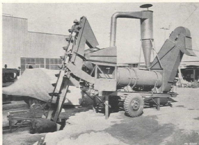
SHALLOW HOLE is dug to accommodate the foot of the cold elevator at the feed end of the machine. Aggregates go through the feeder and are raised by elevator to a hopper above the drier.
