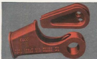
LONG BOWL ROPE SOCKET. Light weight; strong—develops more than 90% of rated cable strength; equal wedging action on all six strands; eliminates crushing and distortion of wire rope.
