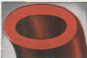
HOLLOW ARCH CONSTRUCTION eliminates excess weight and increases strength. Used on all ESCO buckets over \frac{3}{4} yard. Cast T section arch used on smaller sizes.
