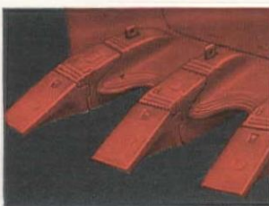
CLEAN CUTTING LIP decreases digging resistance. Tooth holders cast integrally with cutting lip.
