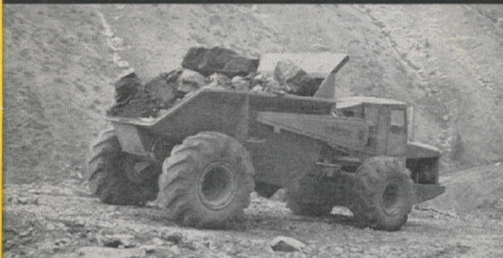
Rock body . . . Here's a typical load of big-chunk rock carried by Tournarockers along Pine Canyon's slopes. 186 h.p. for 16-ton capacity licks the toughest hauling conditions.
