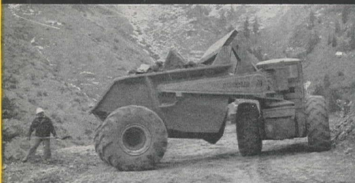
90° turns with positive power steer . . . Short 13' 9" turning radius is an important advantage where operators have to turn and dump their loads along these narrow trails.
