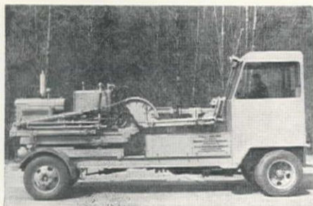
WITH HYDRAULIC cutting attachment folded back over its frame, brush cutting machine goes from job to job at legal road speeds. Cutting bar is held at front of wide vision cab by special bracket.
