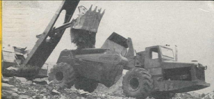
Big target . . . Operator on Goodfellow Brothers' 2-yard shovel has large target with Tournarocker's 12' 5" x 8' top opening . . . speeds shovel swings, has less spillage.
