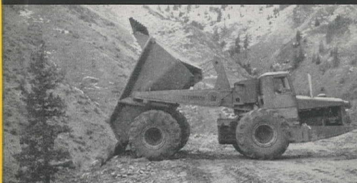
Front-wheel drive . . . Means you can keep the drivewheels of the prime mover on firm ground. Front or rear wheel air brakes can be set independently.
