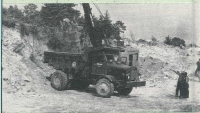
15-ton Rear-Dump ... semi-rigid or spring mounted drive axle.
