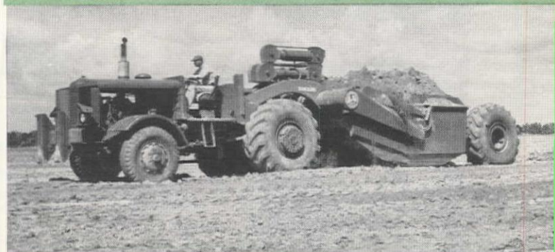
Euclid Scraper picks up a heaped load on an airport job in North Carolina. Capacity is 15.5 cu. yds. struck . . . 275 h.p. diesel engine.
