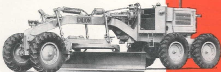
No. 104 MOTOR GRADER Heavy-Duty, 76 h.p. Diesel Engine
