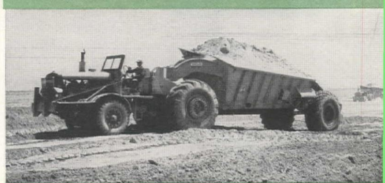
Bottom-Dump Euclids range in capacity from 13 to 25 cu. yds., have diesel engines of 190 to 300 h.p. This "Euc" is hauling approximately 30 cu. yds. at a big earth fill dam in Colorado.
