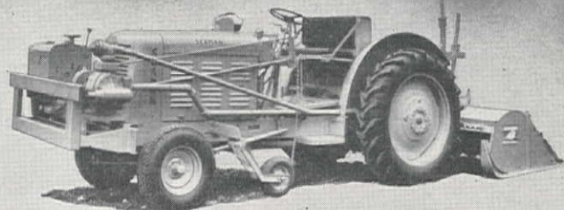
The SEAMAN SELF-PROPELLED TRAV-L-PLANT. Like the Self-Propelled Mixer except for addition of spray bar, pump, pump tachometer fifth wheel assembly and meter for precision control of bitumen or water application. 7 ft. mixing width. Gasoline or diesel powered.
