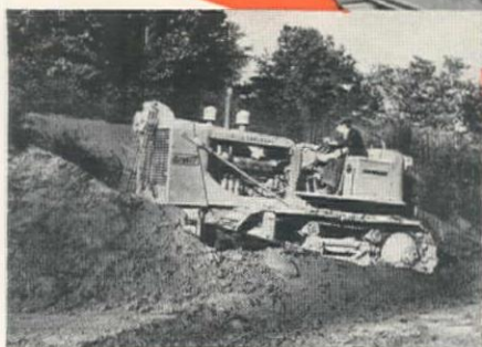
HD-15 —27,500 lbs.—102 Drawbar H.P.—powered by a 6-cylinder GM Series 71 Diesel engine.
