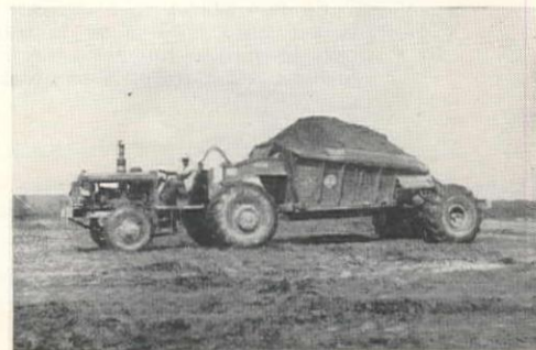
Carrying a heaped load of about 18 cu. yds., this Bottom-Dump hauls overburden at a big open pit bauxite operation in Arkansas. Bottom-Dump "Eucs" are powered by engines of 190 to 300 h.p., have capacities of 13 to 50 cu. yds.
