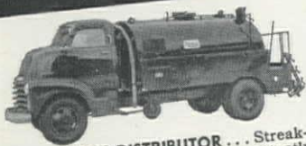
BITUMINOUS DISTRIBUTOR ... Streakless application with pressure constantly and automatically maintained.
