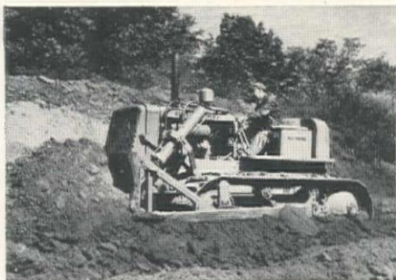
HD-9 —18,500 lbs.—70 Drawbar H.P.—powered by a 4-cylinder GM Series 71 Diesel engine.
