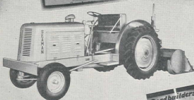
The SEAMAN SELF-PROPELLED MIXER 7 ft. mixing width. Gasoline or Diesel powered.
