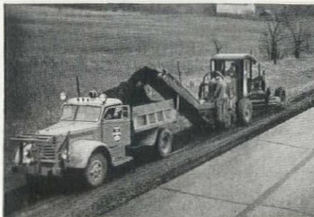
The Loader Attachment solves the ditch and shoulder cleaning problem.
