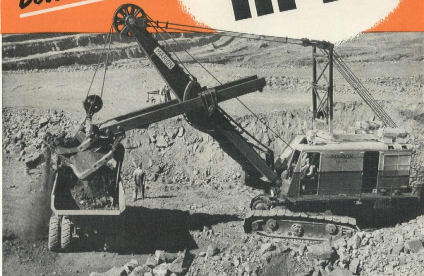
Machine illustrated has Diesel power with electric swing. Also available as full Ward-Leonard Electric machine.
