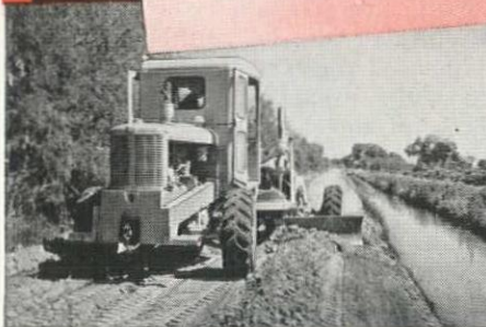
Blading in reverse is easy, thanks to All-Wheel Steer.
