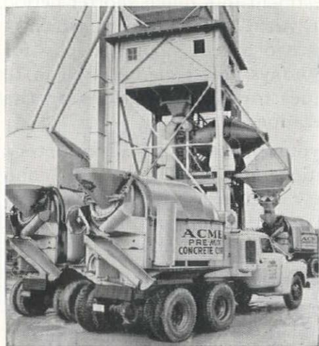
A WINNING COMBINATION — Smith Tilting Mixers for pre-mixing or pre-shrinking concrete and Smith-Mobile Agitators for delivering the concrete to the job.
