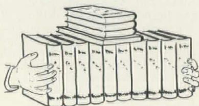
A simple analogy—squeezed together, a "beam" of books can support a load.
