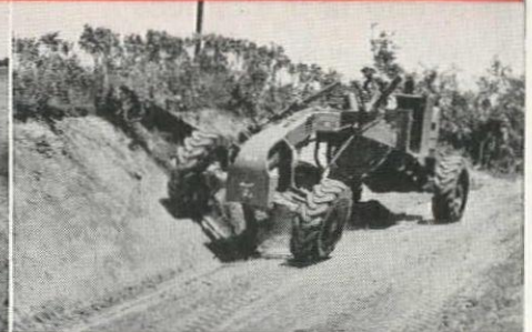
Riding the bank to reach extra high with the 13-foot blade.
