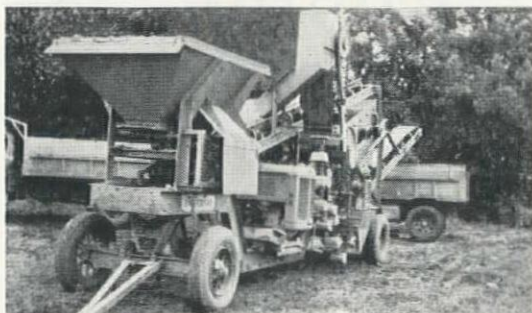
CSE-TRAVELER —Closed circuit plant with bucket elevator return from crusher to screen. Produces specification material. Available in 916, 1016, 1020 or 1024 sizes with bronze or roller bearing jaw crushers.
