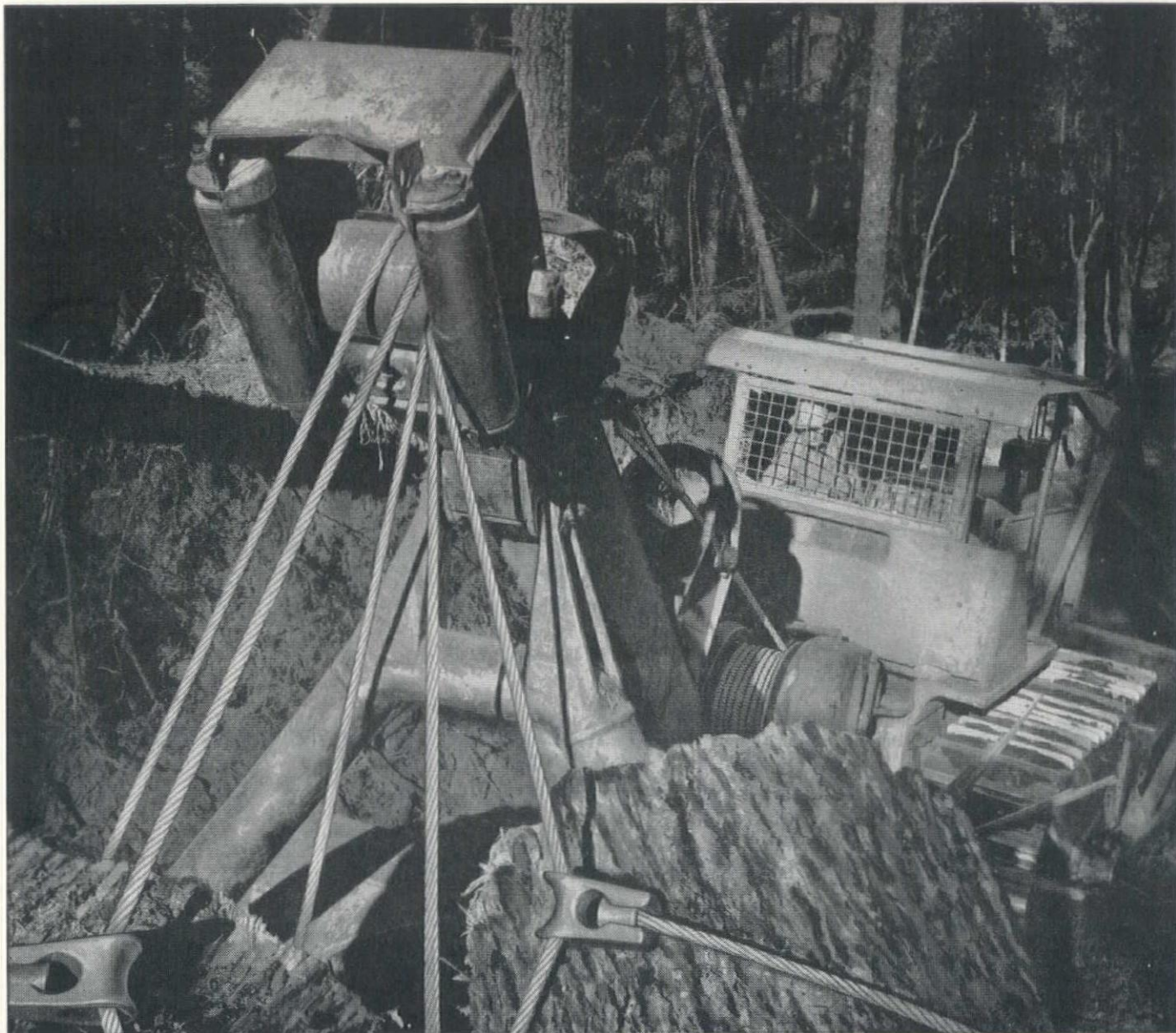
Tractor arch logging using Tiger Brand Wire Rope at Jensen Lumber Co., Willits, California.
