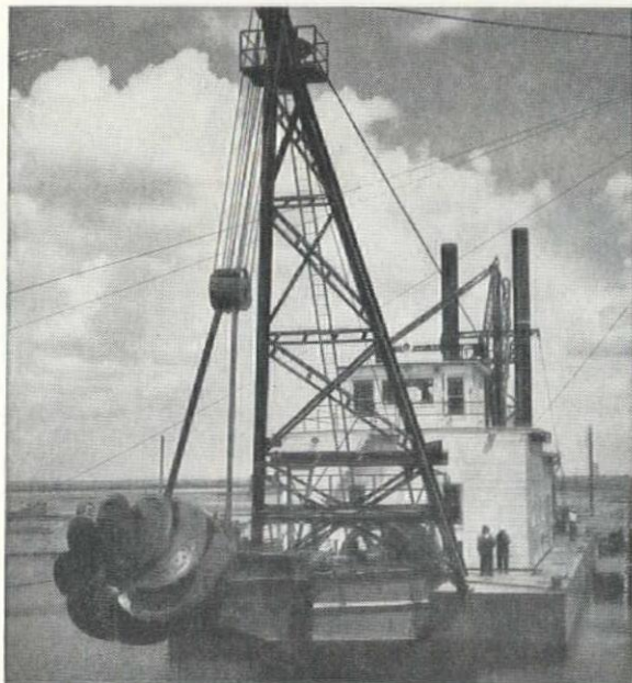
View above shows Bucyrus-Erie hydraulic dredge installation at work. In foreground on floats are electric cables which supply 6600-volt, 3-phase power to the 4000-hp pump motor, 500-hp cutter motor, and various other motors and control. Below is front-view close-up showing cutter in raised position.
