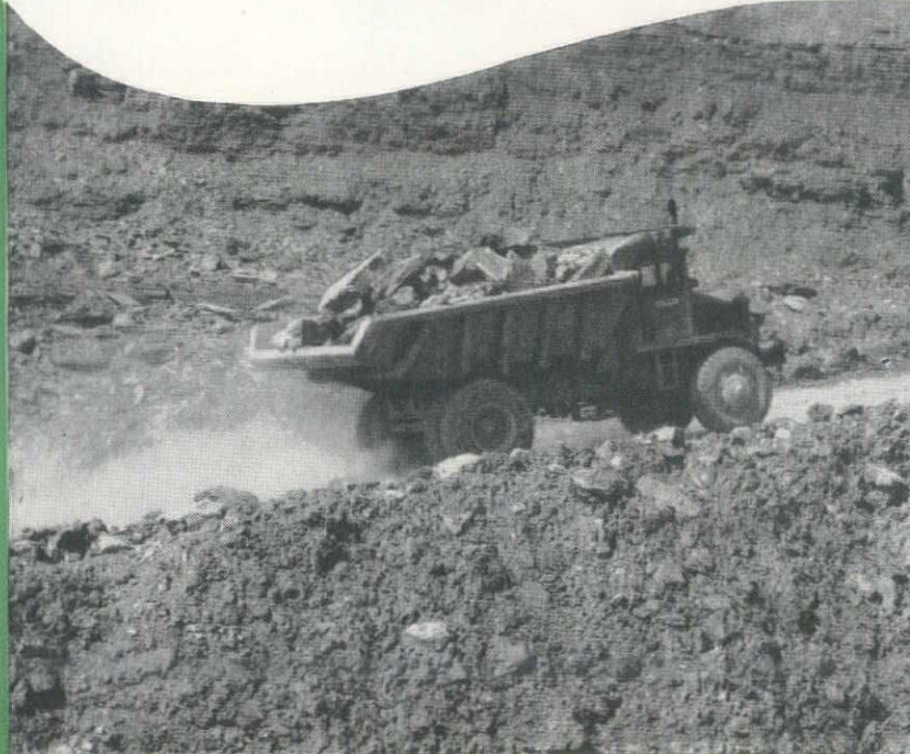
This 15-ton Rear-Dump "Euc" loaded with rock excavation climbs a 10 per cent grade at Bowerston, Ohio. Contractor is Hunkin-Conkey Construction Co.
