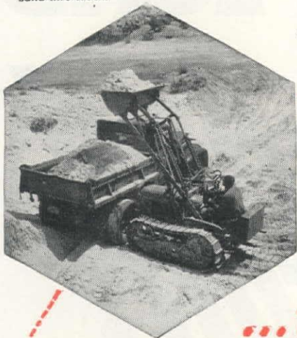
OLIVER HG Crawler Tractor with Ware Loader loading sand into truck.
