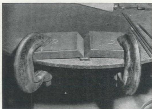
2 Manganese plates beveled and ready to weld.
