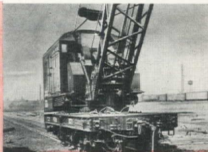
HOISTING —Converted from steam to GM Diesel Torque Converter power—estimated operating savings will pay repowering and overhaul cost in less than two years.
