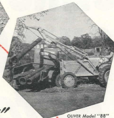
OLIVER Model "88" Wheel Tractor with Ware Boom handling cast iron pipe.
