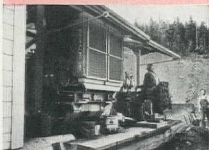
LOGGING —Powered with GM Diesel Torque Converter unit, this Washington Iron Works yarder has yarded 140,000 bd. ft. per day.
