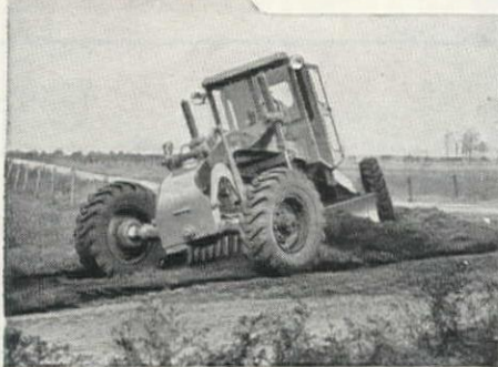
"88-H"—a new model of medium size with all the extra traction and maneuverability of All-Wheel Drive and All-Wheel Steer.
