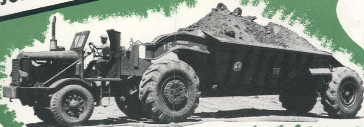
BOTTOM-DUMP EUCLIDS 13 to 25 cu. yd. capacity. Top speeds loaded up to 34.4 m.p.h.
