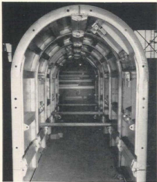
Tunnel form with 4-foot circle, 6 feet deep, built by NOBLE for Campbell-Bennett, Ltd., Vancouver, B. C.
