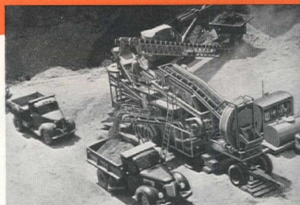
2 TwinDual Gravel King—three stages of crushing, two screens for pits with large boulders
