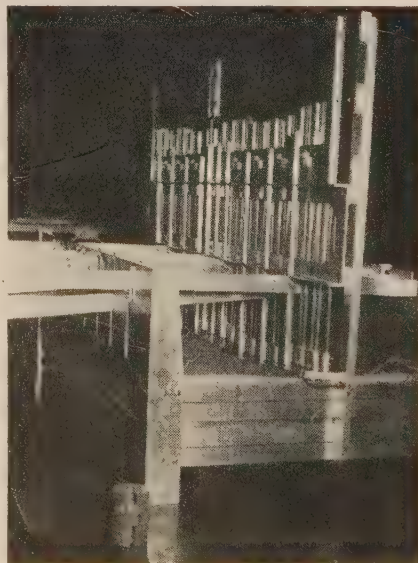
FIGURE 1—Simulated Loads on a Simulated PCC Pavement.
