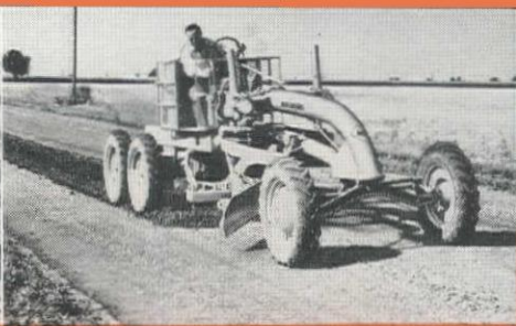
HYDRAULICALLY CONTROLLED SCARIFIER — Located back of circle for greater down pressure. Fast, accurate ripping, controlled penetration. Easy, positive steering resulting from greater front-end stability.
