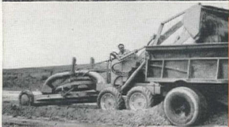
LOADS MATERIAL into trucks with Tractor-motive Loader — from windrows and stockpiles... surplus dirt or snow. Hydraulically operated, simple to mount 5/8 cu. yd. bucket — available with bucket teeth. Note carrying position of loader—no interference with steering or blading.
