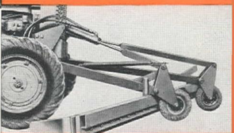
WINDROW ELIMINATOR SAVES TIME. This rear blade saves extra pass by feathering out windrow from grader blade. Means safer traffic conditions, too. Specially designed for the Model D.
