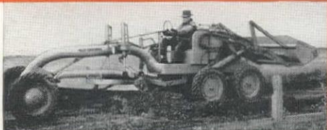
HYDRAULICALLY CONTROLLED SCARIFIER — Located back of circle for greater down pressure. Fast, accurate ripping, controlled penetration. Easy, positive steering resulting from greater front-end stability.
