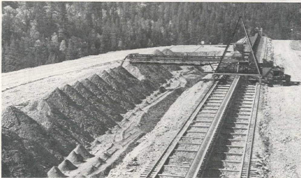
THE SCREENING plant and aggregate storage area. At left are finished product stockpiles. Sand piles on right are, front to rear—medium, coarse and fine. Compare this view with the flow diagram on the opposite page. At right, a general view of the raw aggregate stockpiles and stacker. An underground conveyor carries this material to the screening plant.
