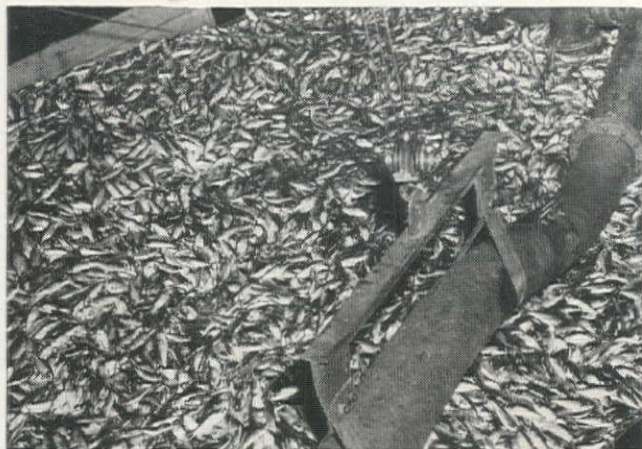
FISHY SUCCESS STORY. The 500,000 fish in this boat were unloaded in less than an hour by a special 12-inch vacuum hose compounded by U. S. Rubber. The hose sucks the fish out of the boat, sends them speeding to a storage bin 1500 feet away.
