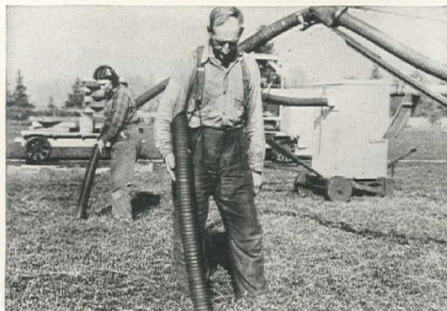
EASY PICKINGS! This vacuum cranberry picker works with great speed, never gets tired. U. S. Rubber made the special hose, aided cranberry growers in developing the machine, thereby increasing the yield.
