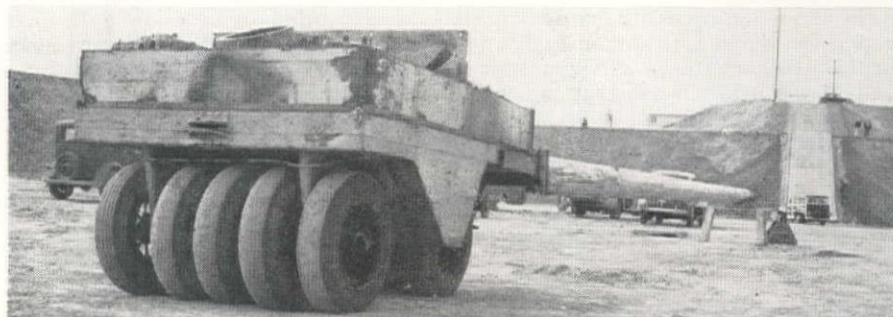
PNEUMATIC-TIRED compactor with heavily cambered wheels and equipped with a 65-ft. gin pole was devised by the contractor for 2:1 slope work on the job. Compartment contains weights.
