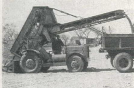
this unit has the solid plate elevating boom mounted on a tractor-type pneumatic-tired chassis. Essentially a stockpile loader, the unit handles all bulk materials. The loader efficiently loads the highest, longest trucks, with a minimum of spotting effort. A welcome design feature is the power-hydraulic
