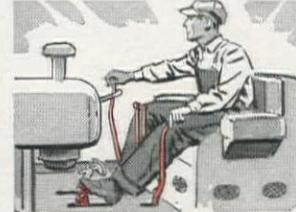
**Separate reverse lever** for quick change of direction. The tractor moves in the direction the lever is moved.
