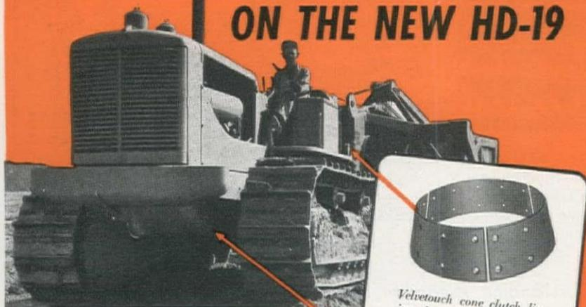
Like other leading manufacturers of heavy duty tractors and earthmoving equipment, Allis-Chalmers specifies Velvetouch for dependable power control. Because the powdered metals, used in making Velvetouch clutch facings and brake linings, are scientifically processed to minimize chattering and slipping... insure smooth, positive action. Genuine Velvetouch lasts longer, too... for it's all-metal... can't rot in oil or "burn" like conventional material. Send for descriptive literature today.
