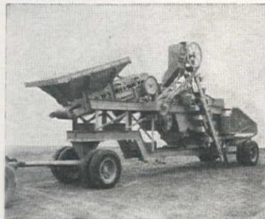
accurately sized material per hour. It is an all-in-one unit made up of standard Cedar-rapids parts consisting of hopper-feeder and feed conveyor; bucket elevator and return conveyor; sand and delivery conveyors, and a choice of four sizes of either plain or roller bearing jaw crushers.
