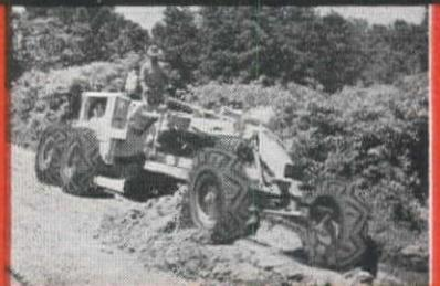
General Tractor Grader Tire with maximum traction from high, long-wearing, self-cleaning tread ribs. No side slip.
