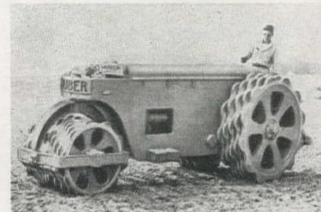
of twelve 4-in. high scallops and the ribs are staggered from one row to another in such a manner that there is a high point every 3½ in. The ribs are 2 in. wide and are spaced 2½ in. apart. The slope of the scallops on one roll is opposite to that on the other roll. Front roll scallops are similar except with less height. The staggered arrangement provides a kneading action that produces better compaction with a minimum of lateral displacement of the soil.
