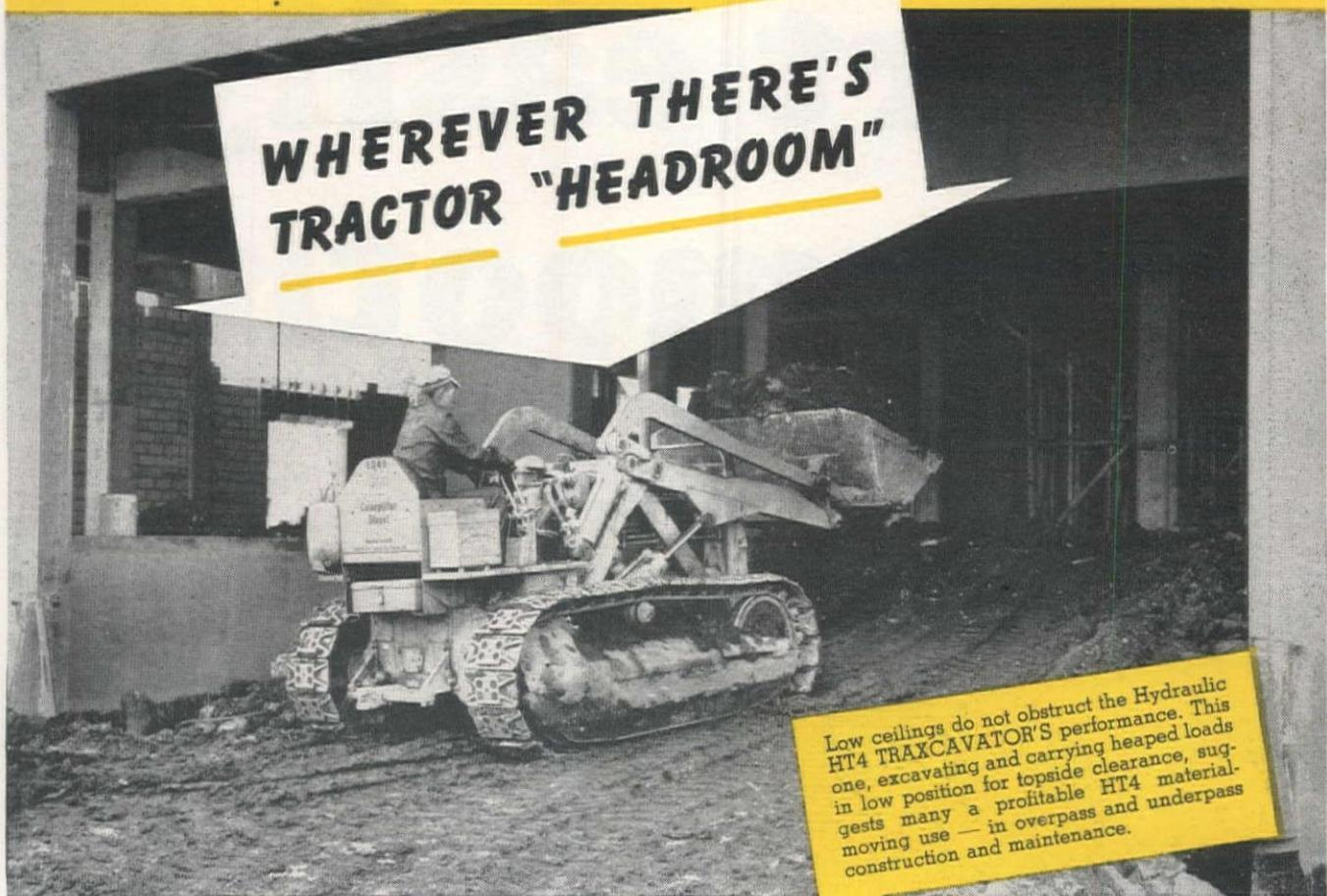
Low ceilings do not obstruct the Hydraulic HT4 TRAXCAVATOR'S performance. This one, excavating and carrying heaped loads in low position for topside clearance, suggests many a profitable HT4 material-moving use — in overpass and underpass construction and maintenance.
