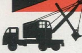
**1/2-YARD.** 205 shovel, pull shovel, dragline, clamshell,  $7\frac{3}{4}$  to 10 ton crane... on crawlers or rubber tire mount.
