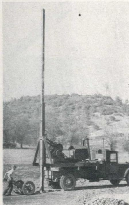
for digging larger or smaller holes. Standard size hole is 28 to 30 in. square. Being truck-mounted, the unit is readily movable over highways, rough terrain, through timber, etc. The digging process is very effective under most conditions, and will operate satisfactorily in water unless extreme caving occurs. In areas where water table can be reached effectively, a large size hole makes an excellent water well.
