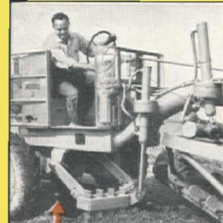
HYDRAULIC SCARIFIER —does a surprising job ... rear-end weight keeps teeth ripping uniformly, at desired depth—smooth, positive steering.
