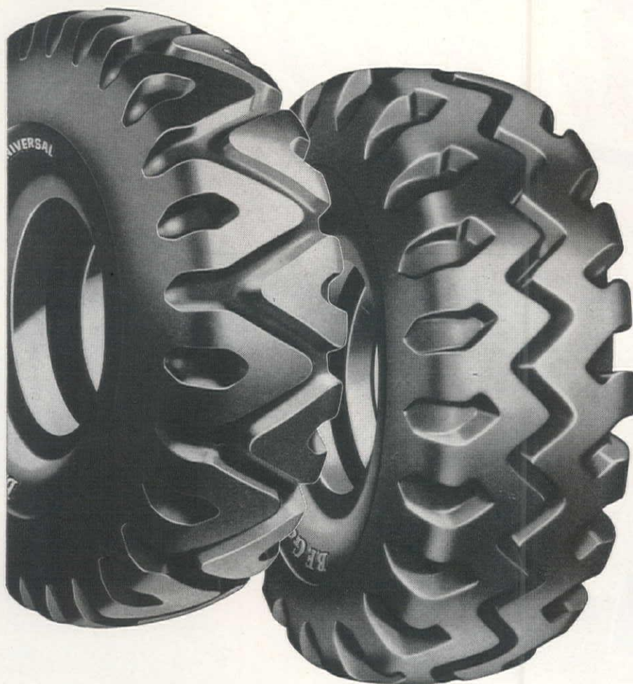
Universal all-nylon for jobs where traction is problem. Note 2-way tread, bulky wedge-shaped cleats.
