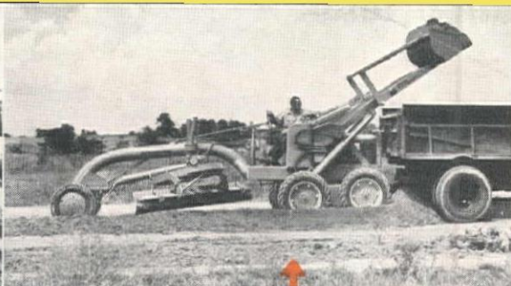
HYDRAULIC SCARIFIER —does a surprising job ... rear-end weight keeps teeth ripping uniformly, at desired depth—smooth, positive steering.
