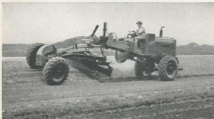
Offsetting the grader through All-Wheel Steer neutralizes side thrust. In the photo above, the rear drivers push behind the "toe" of the blade, the front drivers pull ahead of the "heel." All wheels stay clear of the heavy windrow.
