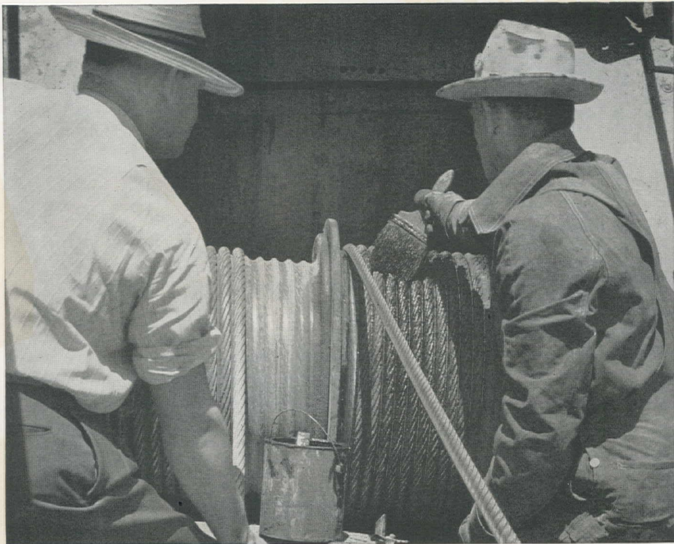
To get top wear, rope should be oiled now and then with a suitable lubricant. Here Columbia's Tiger Brand Field Specialist discusses one method...just one of many of his services to users.
