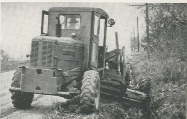
Ditches too wet, or too muddy, to furnish traction for ordinary graders are handled easily by the A-W machine as in the photo above. Rear Steer puts the back wheels up where the "going is good"—but only Rear Steer can do it.
