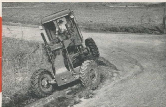
Short radius curves and sharp corners are no problem. Making a ditch cut around the corner shown in the picture above is easy for the A-W operator—impossible with any other grader.
