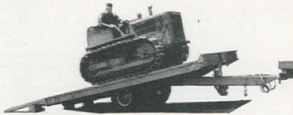
brakes are optional. One feature is the double acting hydraulic ram which cushions the deck when it is being raised or lowered.
