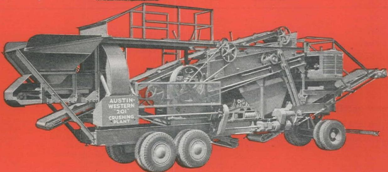
The shovel-loading hopper is fitted with inclined grizzly, and mechanical feeder. All principal units are shaft and V-belt driven. Notice the fully-enclosed brakes.
