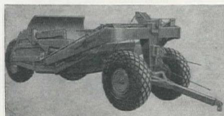
is its interchangeability with the scraper unit S-300 of the TS-300 Motor Scraper. By changing the main frame and tires, if necessary, and the addition of rear wheel brakes, the unit can be hooked directly to the T-300 tractor to make a high-speed, self-propelled unit.
