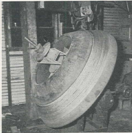
A FOUR-FOOT cone in the process of being hard-faced. It will require 250 lb. of metal.
