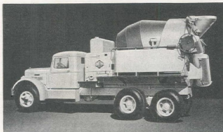
Smith-Mobile 6½ yard Agitator. Loads and discharges at top speed, even dry, low slump concrete. Takes entire batch of a Smith 6 yard Tilter.
