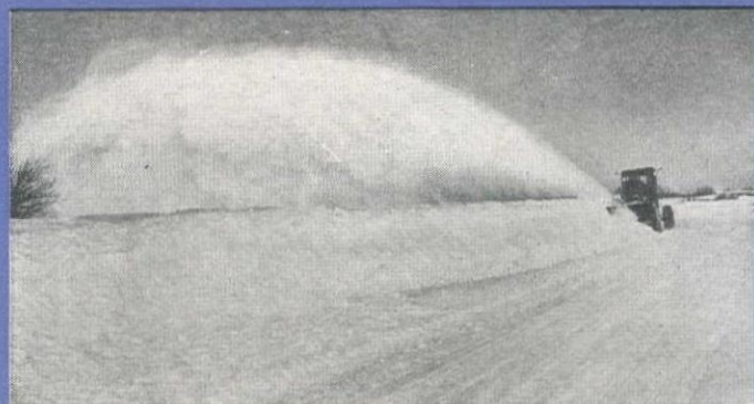
Power and steering control at all four wheels holds the grader steadily to its work in widening.
