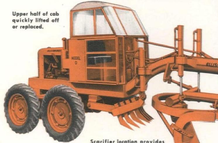
Scarifier location provides extra down pressure and allows controlled steering.
