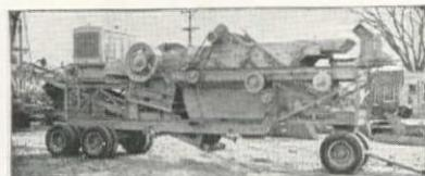
**Cedarapids Scalping Units** consist of a single jaw or twin jaw crusher, horizontal, double-deck vibrating screen with conveyors, all mounted on pneumatic tired trucks. May be used for primary crushing when oversize is not too large, or to follow a portable primary in a quarry. Choice of five sizes.
