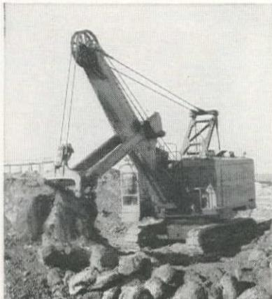
alternator is designed specifically for shovel service with a swing and crowd generator mounted in one frame. Low field current and specially designed magnetic field structure combine to develop faster response to changes of load and control. The new shovel is made possible by P & H's "Magnetorque" Hoist Drive, which eliminates the hoist generator, hoist motor, slip friction clutches and other mechanical devices usually involved in the hoist train.
