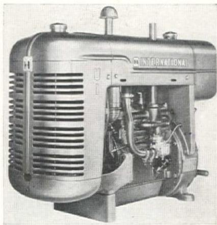
can be equipped to operate either on gasoline or natural gas. Stripped, the U-1 delivers a maximum of 16.3 brake horsepower at 2500 rpm. Overall dimensions: 26½-in. length; 16½-in. width, and 25-in. height. The engine itself weighs 280 lb.; the complete power unit, 450 lb. The engine should be suitable for powering fans or blowers, oil or water pumps, generators, portable in-plant or outdoor units, etc.
