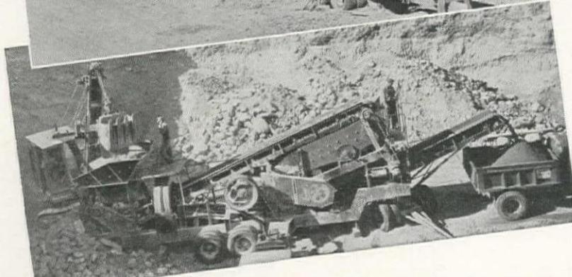
*Left, top:* A Bin-loading Telsmith Dual Portable with field conveyor, owned by Colonial Construction Co., Spokane, Wash.
