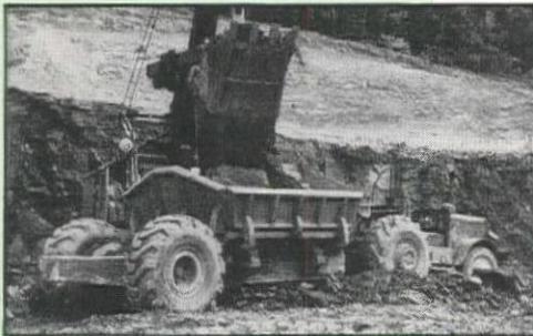
Low, wide hopper speeds loading and reduces spillage at an open-pit coal mining operation in West Virginia.
