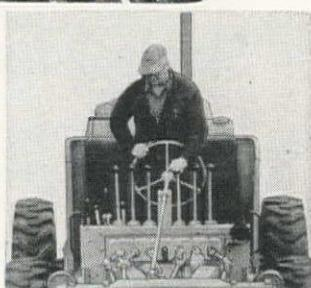
**1** Positive Mechanical Control System Provides Fast, Accurate Blade Adjustments.
