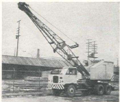
type truck frame that is reinforced the full length of the carrier. The method of attaching the crane lower base to the carrier permits the transmission of loads evenly
