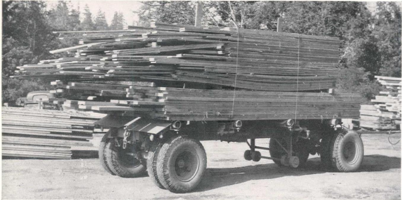
Clark Coffelt & Son of Arcata, California are lumber haulers for Addison & Sons Lumber Company of Maple Creek. The haul is 30 miles over county roads with about 7 miles of adverse grade. The truck and trailer make two trips per day over the narrow winding road, hauling from 12,500 to 13,000 board feet of fir on each trip.
