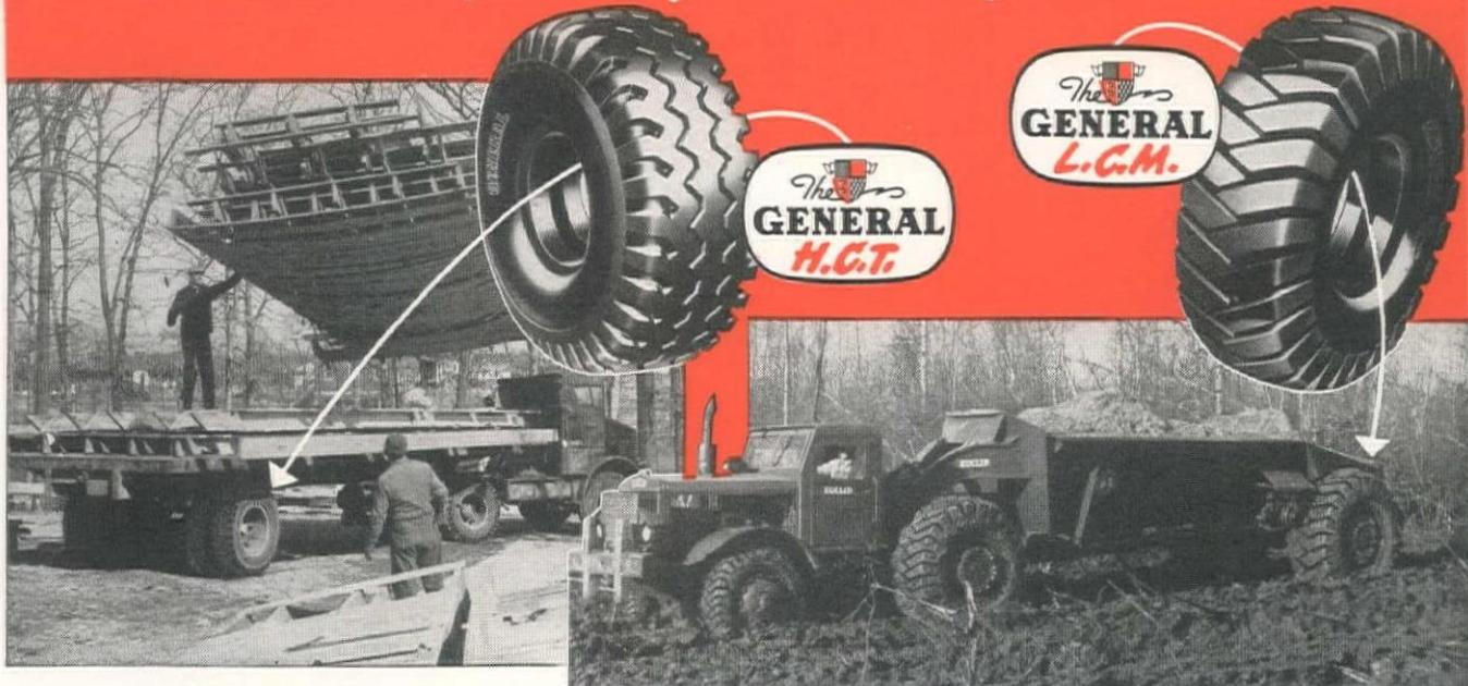
The *General H. C. T.* Truck Tire is designed with a deep, zig-zag tread that disperses loads over more of the stronger carcass. Tremendous rubber lugs form wide, sturdy reinforced shoulders. Through off-the-highway sand, gravel and mud, out and over-the-road the *General H. C. T.* delivers the load faster, safer, at lower cost. More rubber, more strength for more original miles—more dependable recap miles.
