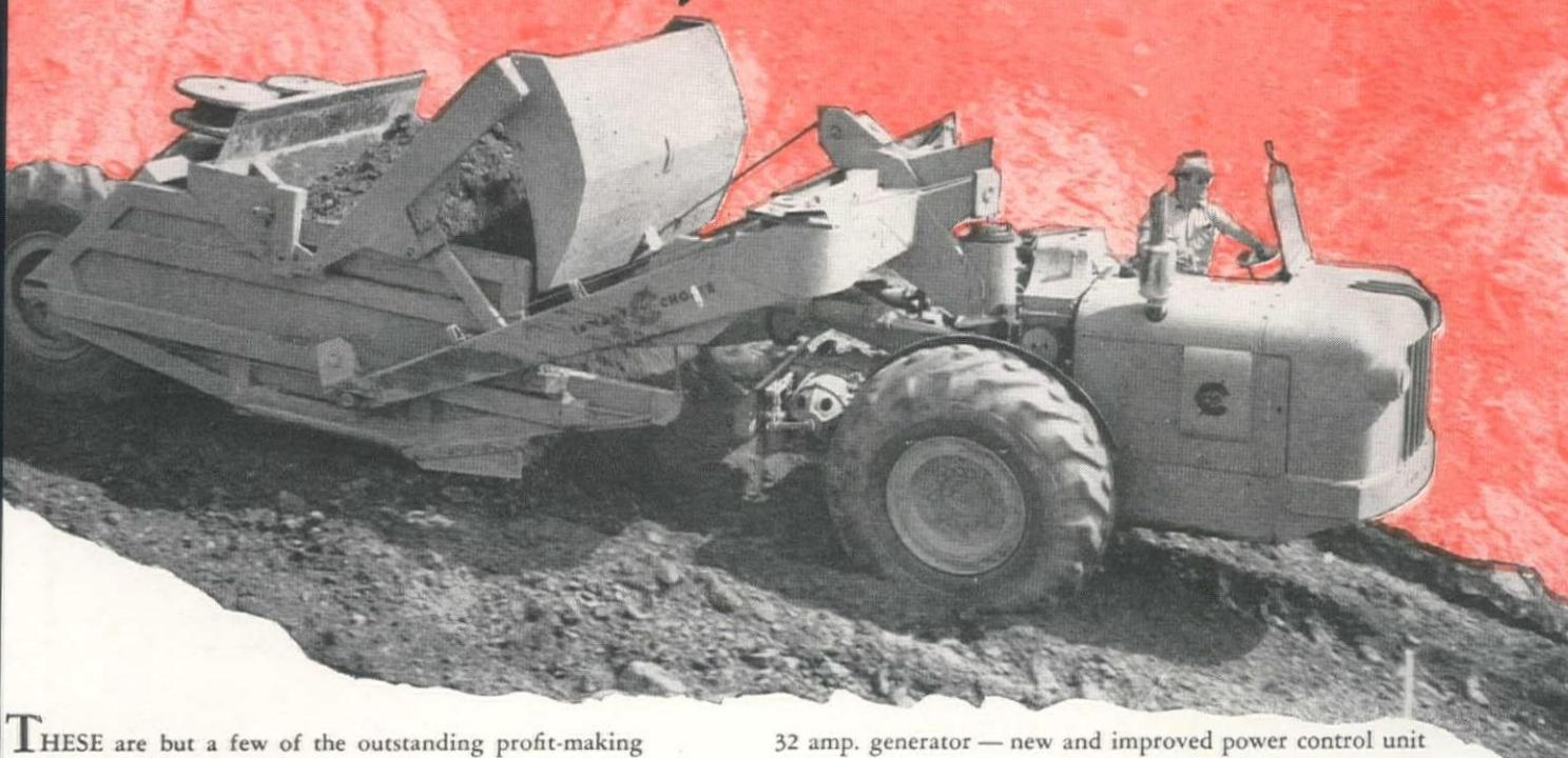
THESE are but a few of the outstanding profit-making advantages of the LPC Motor Scraper which let you carry 17½ heaped yards each trip, even in the heaviest materials. Higher speeds mean more trips per hour — per day — per year.
