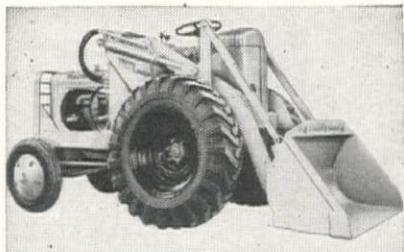
bucket down and narrow width of 5 ft. 9 in. means the unit is small enough to be used where working areas are limited. Close-quarter operation is possible since the bucket is eased into the material and picks up a load through forward crowding action and an automatic "tilt-back" feature. The bucket is hydraulically operated.
