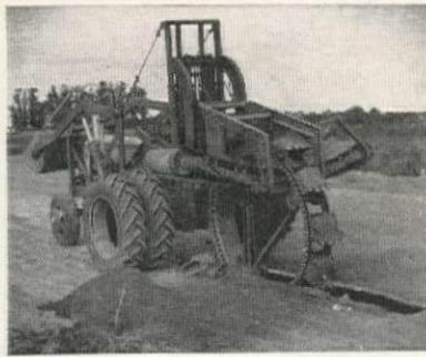
Features claimed: The trencher has eight forward creep speeds and two wheel speeds to provide 16 forward digging combinations, and is especially profitable for foundations, drainage ditches, water and service
