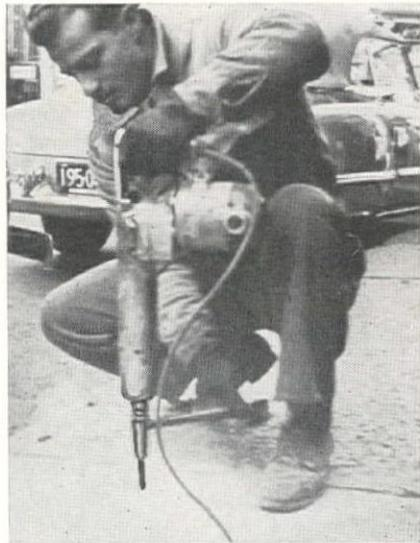
mer, and is available in sizes from 3/16 to 1 in., inclusive, with suitable chucks that fit the drill. Reports from users drilling hard concrete show expense for bits reduced from 14 to less than 2 cents per hole.
