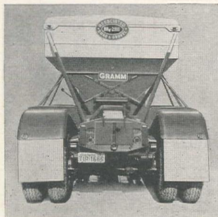
Direct truck chassis mounted aerated units used by International Cementers, Inc., Long Beach, Calif., as front unit of 4-wheel trailer train.
