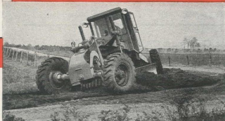
"88-H" Ditching around short radius curves is easy for an "88" or "99"—impossible with any other grader.
