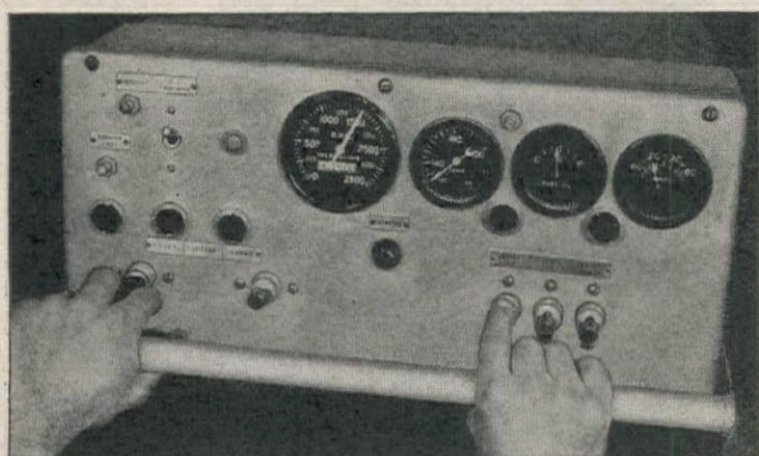
Control panel of LeTourneau's Model "C" Tournapull; a fingertip movement instantly applies power to motors which steer the vehicle, operate hoist, apron or tailgate.
