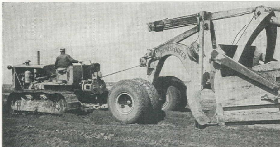
POWER WINCH and electrically-operated power control unit used on Lewis & Queen's LeTourneau Carryall scraper, above, was recently developed by Kay-Brunner Steel Products, Los Angeles.
