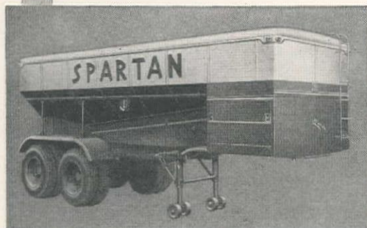
Gramm aerated bulk cement trailers used for field transport and storage of oil well cement. Ruggedly built for off-highway service.
