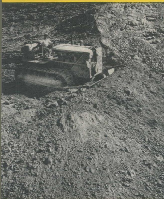
This two-fisted "Caterpillar" Diesel D8 Tractor has front-end cable control for the "Caterpillar" No. 8A Bulldozer, and a 2-drum rear control for scraper use.
