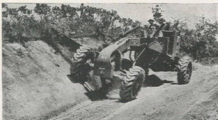
"99-H" All-Wheel Drive and Steer make it possible to slope banks beyond the reach of any other grader.
