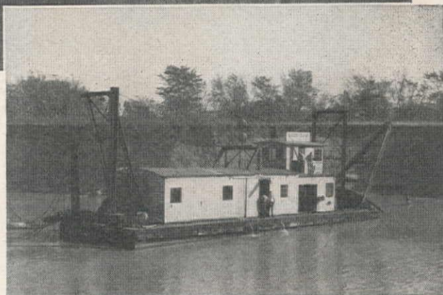
Kershaw Mining Co.'s dredge "Chickasaw" pumping aggregate (45% gravel, 55% sand) on the Illinois River. Amsco type XH 15" pump is used.
