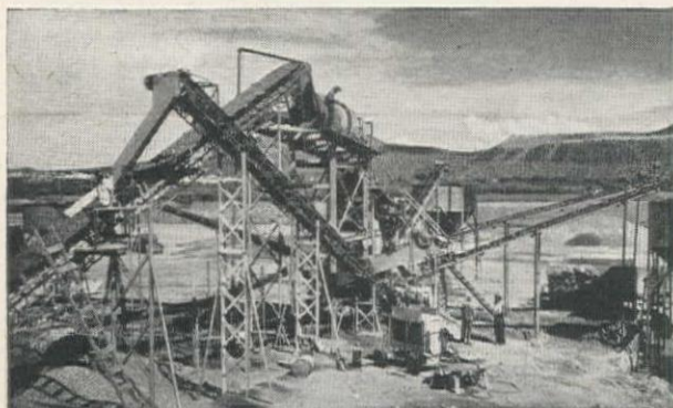
Crushing screening and washing plant with primary jaw crusher, secondary roll crusher, scrubber classifier, conveyors, and bins.
