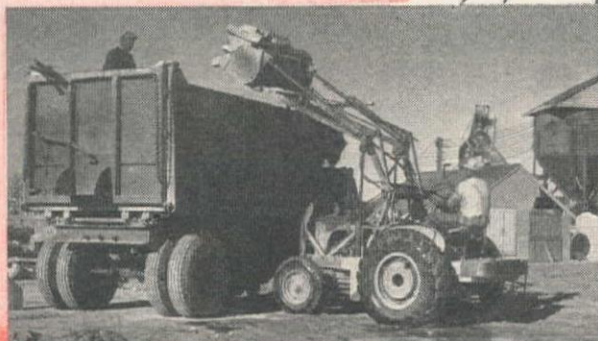
Model "SI" with hydraulic shovel loader handling crushed rock in Wisconsin. In large picture, with sheepfoot roller, is Model "LAI."
