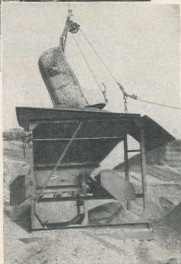
The portable feeder-hopper unit has a 36" x 6' Telsmith Heavy-Duty Plate Feeder.
