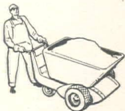
Bucket holds 1000 pounds of wet or dry material
