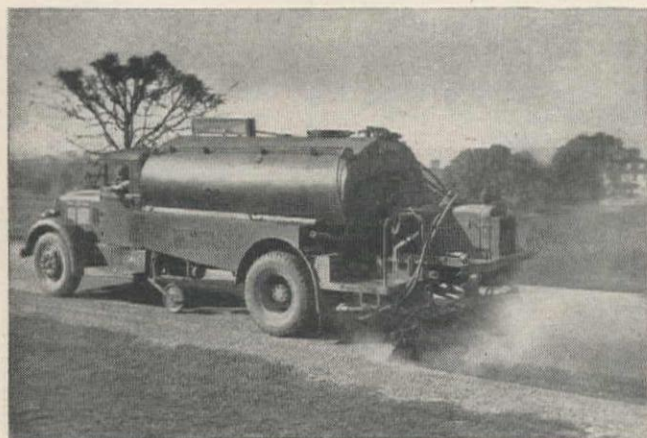
One-man controls, when desired, make it possible to operate Etnyre distributors from the cab, eliminating rear platform man, cutting labor costs.
