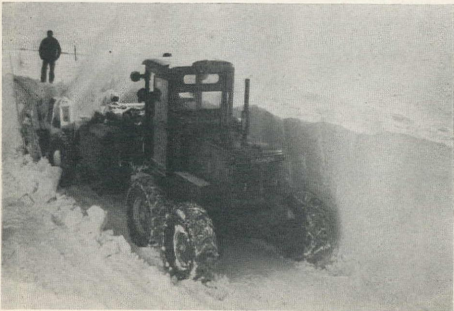
COLORADO was hard hit by the winter snows too. Below, a state-owned Adams Model B-70 Rotary widens a cut previously opened on a road in Weld County, Colo.
