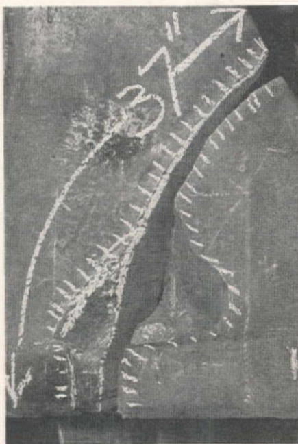
TWO-INCH CUT completely through the skeg, left, was made prior to welding. Completed thermit weld, right. Ship was floated just 25 hr. after the weld was applied.
