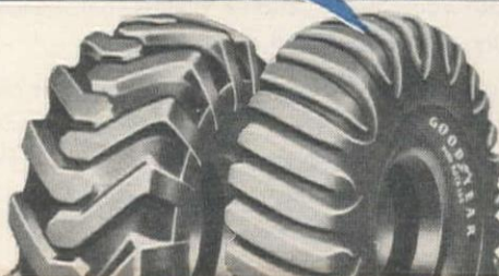
EARTH MOVER SURE-GRIP for maximum traction on drive wheels
