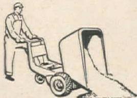
Mechanically dumped . . . operates by foot pedal
