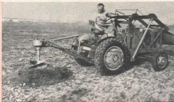
Holes for posts or plantings are dug in a jiffy with earth auger mounted on the Model "VAI."
