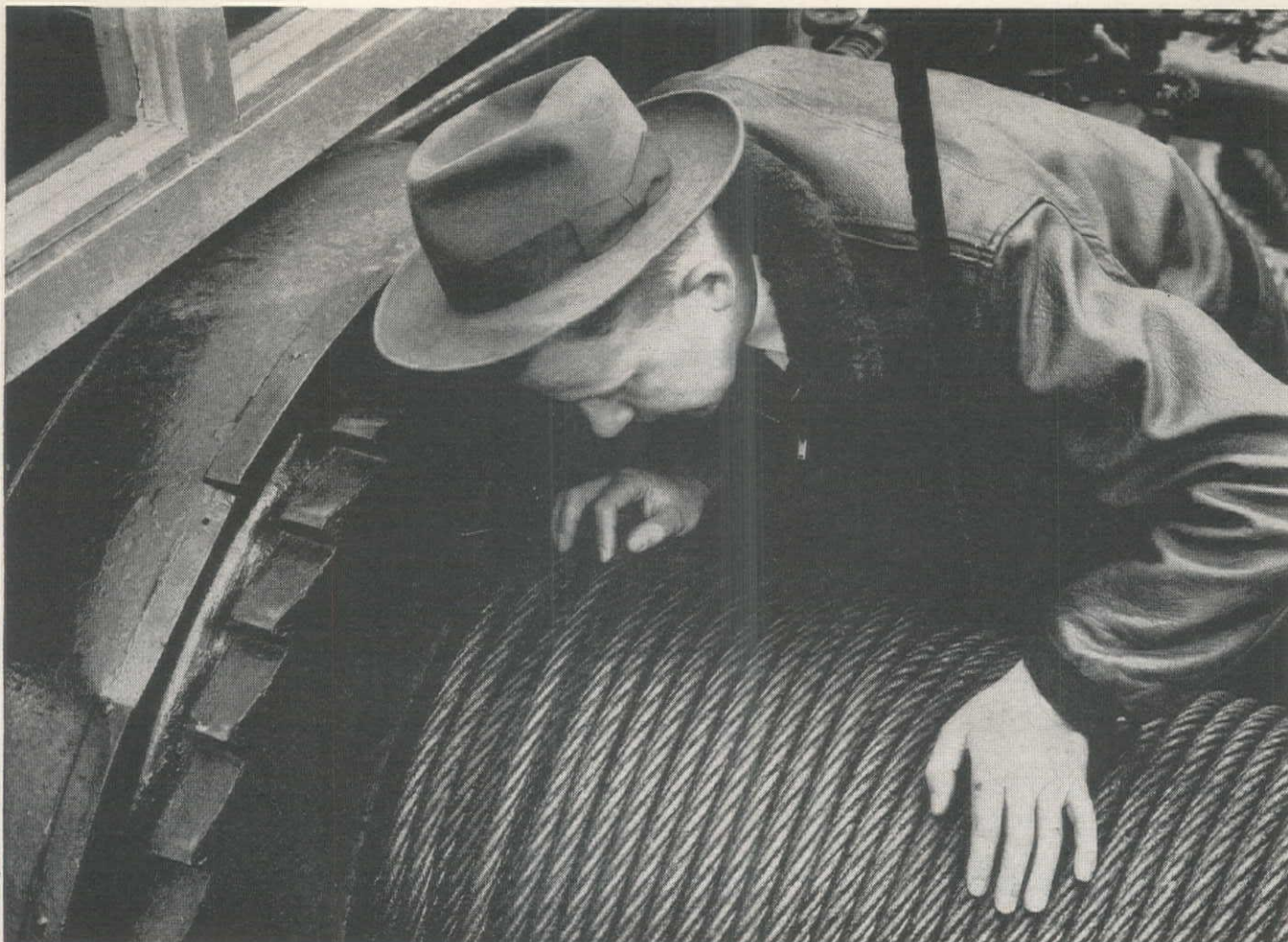
TIGER BRAND Field Specialist is shown here checking a cross-wind on a drum as part of equipment check to insure proper wire rope application. Even such a small cross-wind as this can cause unnecessary abrasion and reduce life of the rope.
