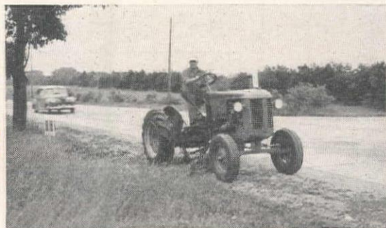
This "VAI" tractor is equipped with scarifier, scraper, and loader—a complete earth-working outfit.
