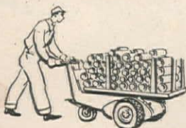
9-square-foot steel platform takes half-ton loads
