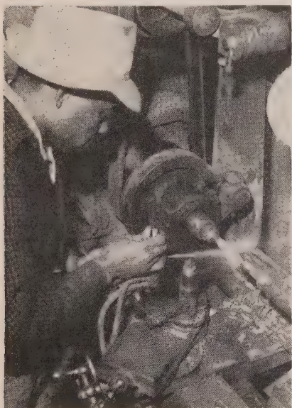
A LATHE SETUP, above, is used to rotate a small shaft during the process of spraying it with molten steel. Such rotation facilitates the application of uniform coatings. Phantom view of the wire-type metallizing gun, below. The white line through the center denotes the wire-feed channel where the alloy is melted and atomized.
